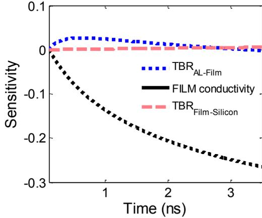
Fig 2 Plot of sensitivity coefficients for  $k_{film}$ ,  $TBR_{Al-film}$  and  $TBR_{film-Si}$  showing that the measurement is sensitive to the superlattice film conductivity and TBR at the Al-film interface, and insensitive to the TBR at the film-silicon interface.
