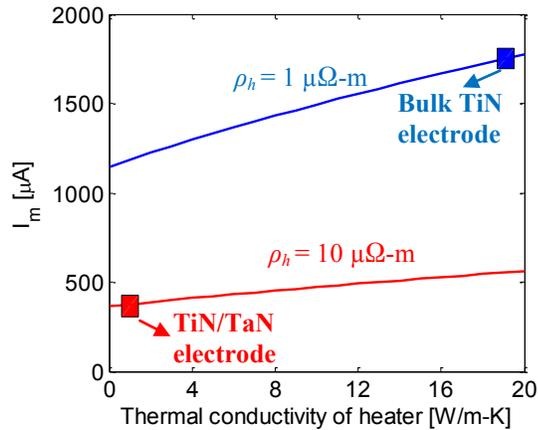
Fig 6 Melting (RESET) current predicted by the simplified thermal model for two cases of heater resistivity (blue:  $\rho_h = 1 \mu\Omega\text{-m}$  and red:  $\rho_h = 10 \mu\Omega\text{-m}$ ). The blue and red squares represent the cases corresponding to bulk TiN ( $k_h \sim 19 \text{ W/m-K}$ ) and superlattice TiN/TaN electrodes ( $k_h \sim 1 \text{ W/m-K}$ ), respectively.
