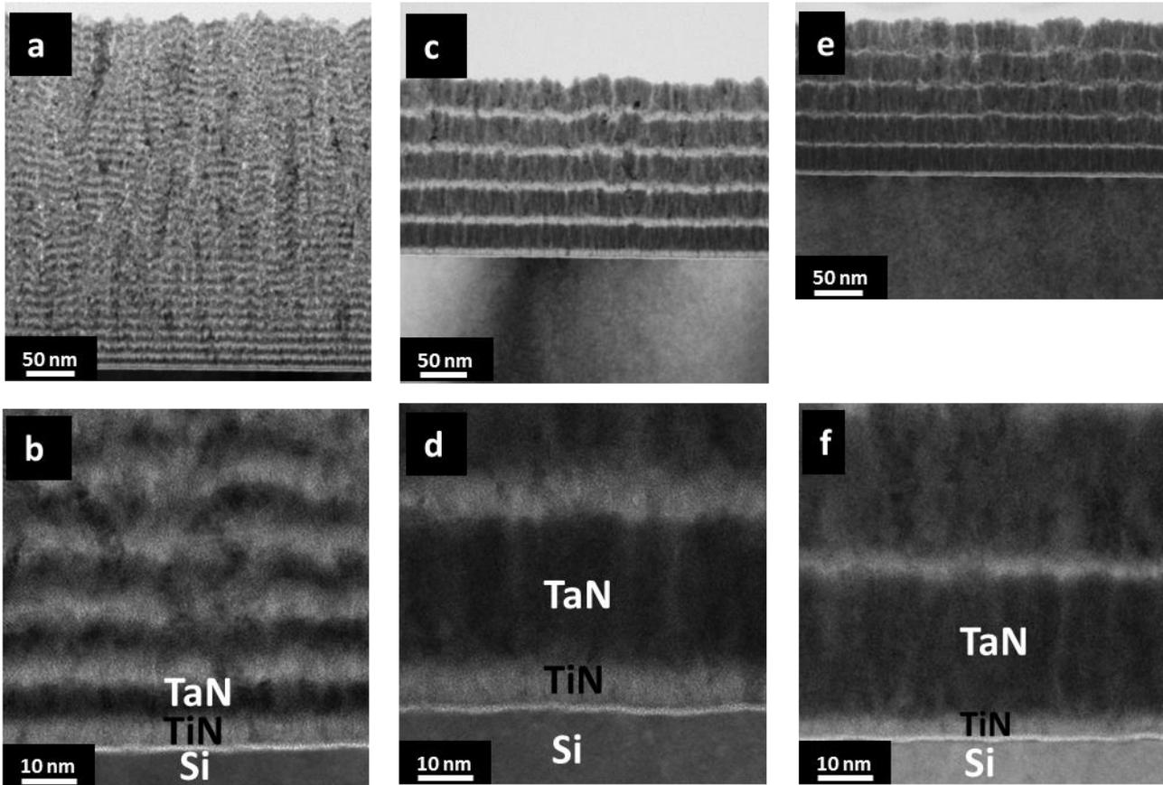
Fig 4 Cross sectional TEM images for (a, b) Sample 1, (c, d) Sample 2, and (e, f) Sample 3. The images in the bottom row are taken at a higher magnification.
