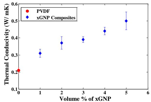
Figure 5: Thermal conductivity of PVDF-xGNP composites.
