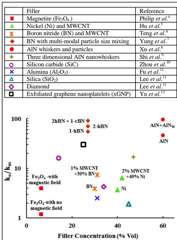
Figure 1. Past data for the thermal conductivity enhancement for various filler materials from literature as a function of total filler volume fraction. The chart lists the different filler particles used in the composites, a subset of which are indicated directly on the plot where efficient percolation pathways are established.
