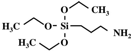
Figure 3. Molecular structure of (3-Aminopropyl)-triethoxysilane used in surface modification of AlN particles for effective thermal coupling with PVDF matrix.
