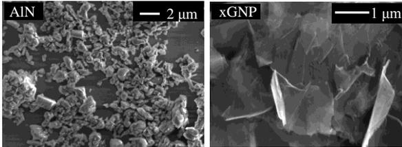
Figure 2. SEM images of AlN and xGNP particles showing particle shapes and sizes.
