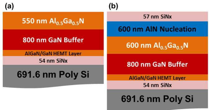
Fig. 2: Cross sectional schematic drawings of the flipped-epitaxial samples for (a) AlGaN transition layer and (b) AlN nucleation layer.
