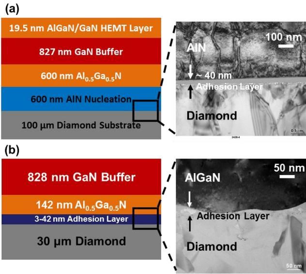
Fig. 1: Cross-sectional schematic drawings of the GaN-on-diamond substrates with representative cross-sectional TEMs near the adhesion layer: (a) 1<sup>st</sup> generation with a 1200 nm-thick Al<sub>0.5</sub>Ga<sub>0.5</sub>N/AlN transition layer and (b) 2<sup>nd</sup> generation with a significantly reduced transition layer.
