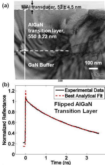
Fig. 3: (a) Representative cross-sectional TEM and (b) thermal trace with data fit for flipped AlGaN transition layer.
