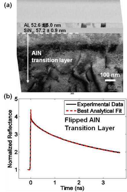
Fig. 4: (a) Representative cross-sectional TEM and (b) thermal trace with data fit for flipped AlN transition layer.
