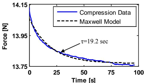
Fig. 10: Stress relaxation curve and corresponding Maxwell model fit. The Maxwell model is adapted to CNT films, which exhibit viscoelastic behavior similar to polymers.
