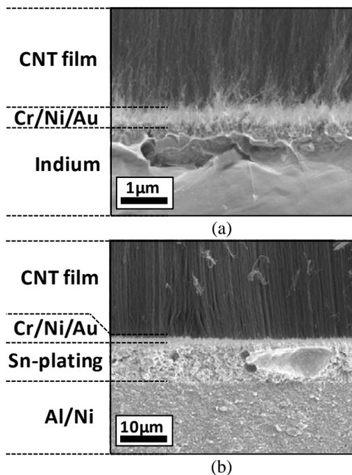
Fig. 2: (a) SEM of indium foil soldered to a metalized CNT film and (b) SEM of NF with Sn-plating welded to a metalized CNT film.
