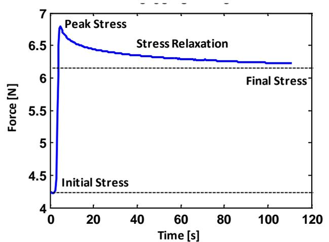
Fig. 9: Viscoelastic stress relaxation of CNT film under constant axial strain. A compressive strain is applied to the film, raising the stress from an initial state to a peak state. Under constant strain, the CNT film relaxes from its peak stress to a final steady state value.
