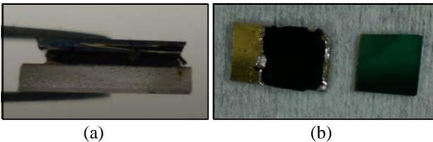
Fig. 5: (a) CNT film is bonded to a fused silica substrate with original growth silicon substrate still attached. (b) Since the indium and NF bonds are stronger than the CNT adhesion to the growth substrate, the silicon can be pulled away.
