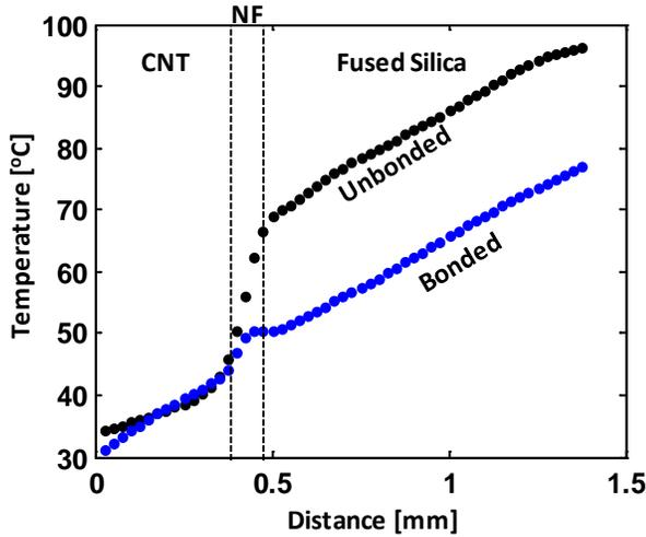
Fig. 7: Comparison of interface temperature drop across a NF bonding layer before and after bonding. Since the temperature drop is reduced, the maximum temperature on the hot side is lower after bonding.
