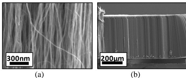
Fig. 1: (a) Scanning electron micrograph (SEM) showing vertical alignment of individual CNTs within the film. (b) SEM of an un-bonded 500  $\mu\text{m}$ -thick vertically-aligned CNT film.
