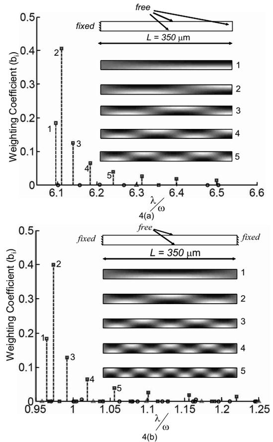
FIG. 4. Thermal mode contributions to lost work in (a) a cantilever and (b) a fixed-fixed beam. The inset shows a sample of significant thermal modes and their corresponding spatial distribution. The dark shaded regions correspond to temperatures higher than the reservoir temperature and the bright regions correspond to temperatures lower than the reservoir temperature.
