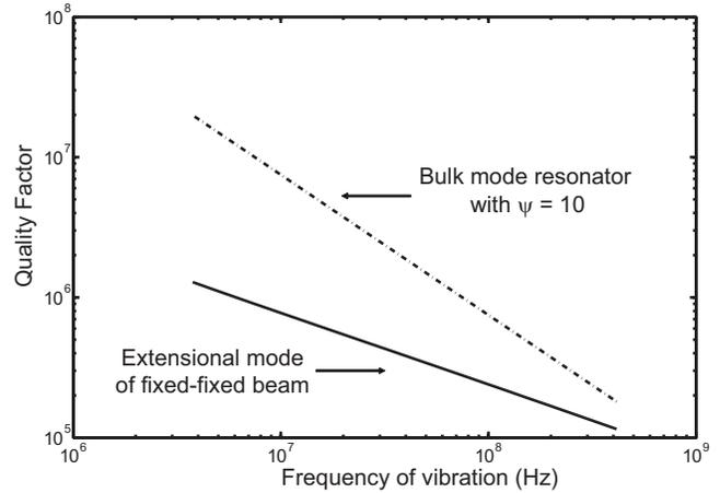
FIG. 3. Quality factor of a fixed-fixed beam vibrating in extensional mode and its comparison with a bulk mode resonator whose quality factor has a frequency dependence as given by Eq. (23) with  $\psi = 10$ . This value of  $\psi$  is close to that for most of the bulk mode resonant modes discussed in this paper.
