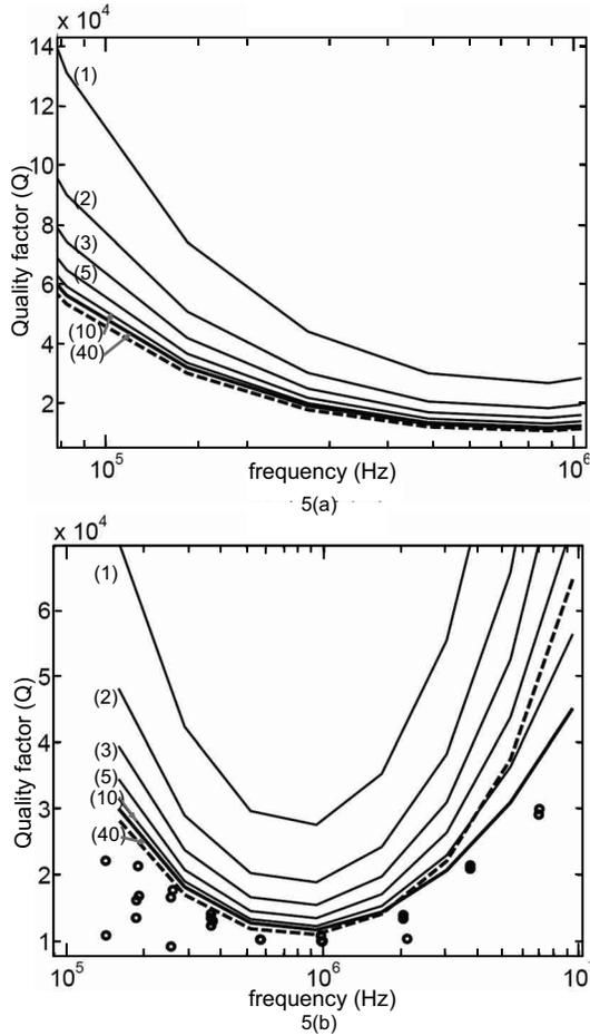
FIG. 5. Quality factor of (a) a cantilever and (b) a fixed-fixed beam. The dashed line corresponds to Zener formula based prediction. The solid lines depict the quality factor when the number of significant thermal modes contributing to the energy loss is equal to the number included next to the line. It can be seen that progressive inclusion of thermal modes finally converges to a value close to that predicted by Zener's formula. The circular markers in Fig. 3(b) represent actual measured data.
