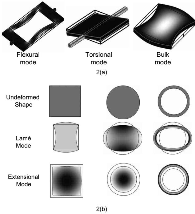
FIG. 2. (a) Three types of mechanical resonators: flexural mode, torsional mode, and bulk mode. (b) Bulk mode resonators with different geometries and mode of operation.
