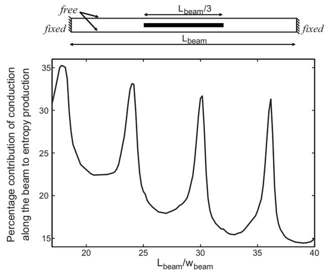
FIG. 7. Longitudinal heat transfer contribution to entropy generation in a fixed-fixed beam with a center slot as shown in the inset figure. In this case, there is significant contribution of lateral heat transfer as well as longitudinal heat transfer to entropy generation making it impractical to amend Zener's formula to assess quality factor.
