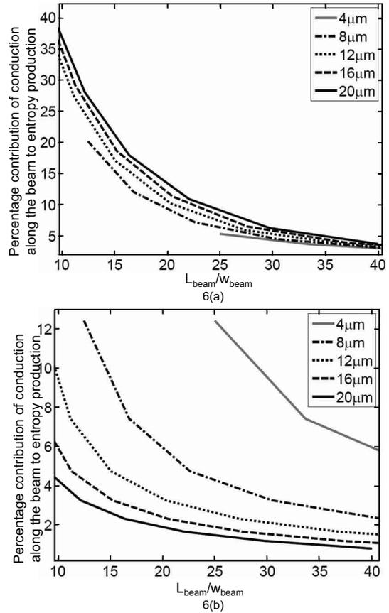
FIG. 6. Longitudinal heat transfer contribution to entropy generation in (a) cantilever and (b) fixed-fixed beam. The approximation of predominant heat transfer across the beam is worse in a fixed-fixed beam as compared to a cantilever. For  $L_{beam}/w_{beam}$  value of less than 20, the contribution of heat transfer along the beam is greater than 10% in the case of a fixed-fixed beam.
