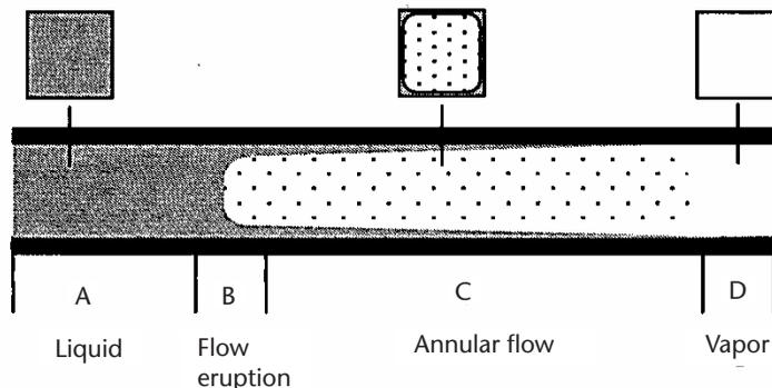
**Figure 10.6** Two-phase flow regime used in the development of the homogeneous flow model by Koo et al. [29]. The flow structure consists of a homogeneous core composed of a mist of liquid droplets and vapor moving at the same velocity, surrounded by a very thin, slow-moving liquid film.
