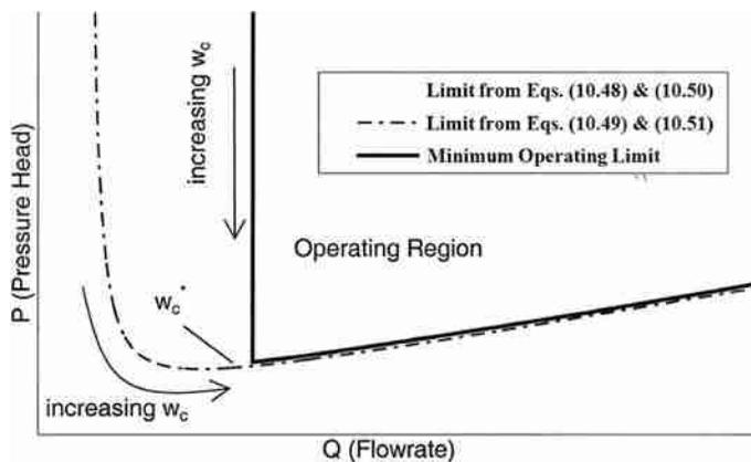
**Figure 10.8** “Operating region” of a microchannel heat sink for a set of given thermal constraints. This map is constructed by plotting and combining the pressure-flow requirements, given maximum-temperature-gradient and maximum-temperature constraints for the microchannel heat sink [39, 40].
