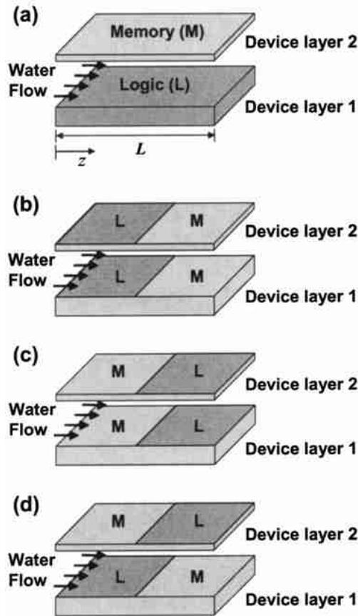
**Figure 10.13** Two-layer 3-D circuit layouts for evaluating the performance of microchannel cooling. The areas occupied by memory and logic are the same, and the logic dissipates 90% of the total power consumption [32].
