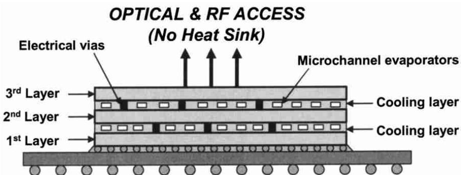
**Figure 10.12** 3-D IC with integrated microchannel cooling system consisting of three device layers and two microchannel layers arranged in an alternating pattern used in the study by Koo et al. [32]
