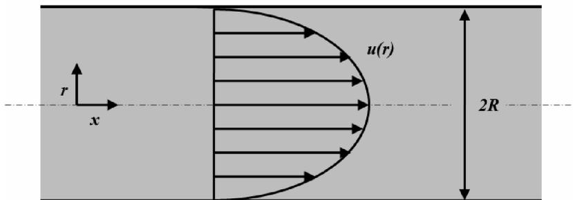
**Figure 10.1** Parabolic velocity profile for fully developed laminar flow in a circular cross section tube. The pressure drop balances the shear stress at the wall, which is constant for fully developed flow and proportional to the velocity gradient at the wall.
