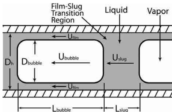
**Figure 10.7** Two-phase flow regime used in the development of the separated flow model by Garimella et al. [36]. The slug/bubble flow regime is considered periodic, and a unit cell consists of a cylindrical bubble surrounded by a uniform annular film of liquid. The bubble/annular film section is bounded by liquid slugs on either side, with the bubble moving faster than the slugs.
