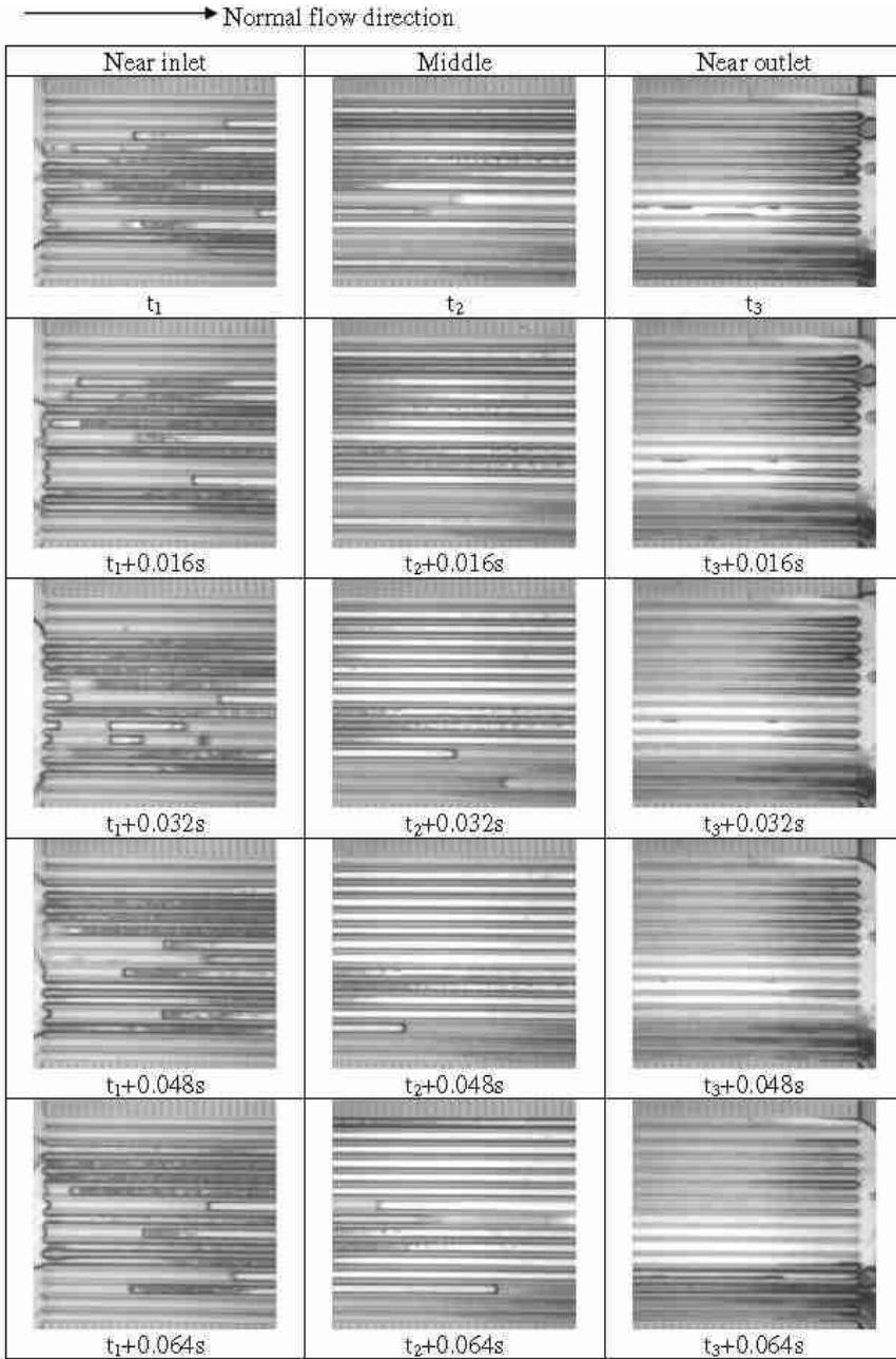
**Figure 10.4** Evolution of two-phase flow patterns in the entrance, middle, and exit regions of a heat sink consisting of 15 parallel microchannels of rectangular cross section 100  $\mu\text{m}$  in width and 70  $\mu\text{m}$  in depth. In this unstable case, forward or reversed slug or annular flows appear alternately in every channel. Intermittent reversed flow of the two-phase mixture to the inlet chamber is also observed [27].
