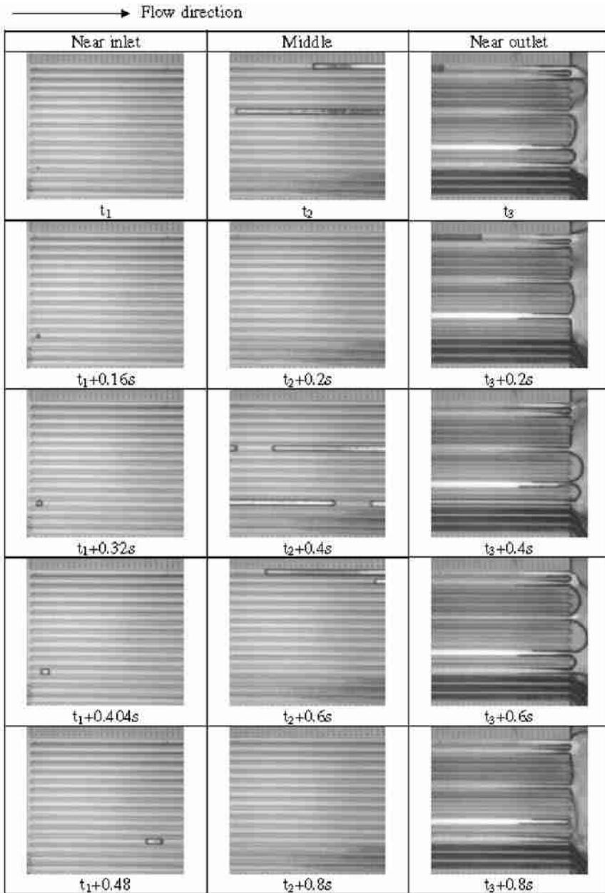
**Figure 10.3** Evolution of two-phase flow patterns in the entrance, middle, and exit regions of a heat sink consisting of 15 parallel microchannels of rectangular cross section  $100\ \mu\text{m}$  in width and  $70\ \mu\text{m}$  in depth. In this stable two-phase flow, oscillations, bubble nucleation, slug flow, and annular flow appear sequentially in the flow direction [27].
