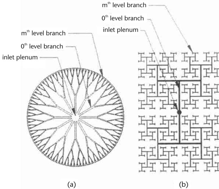
**Figure 10.14** Fractal-like branching microchannel networks in heat sinks used in the study of Pence [48].
