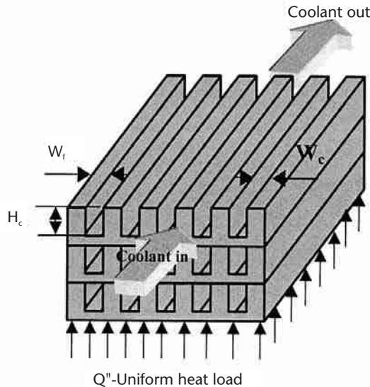
**Figure 10.11** Schematic of a three-dimensional microchannel stack used in the optimization study of Wei and Joshi [41, 42].
