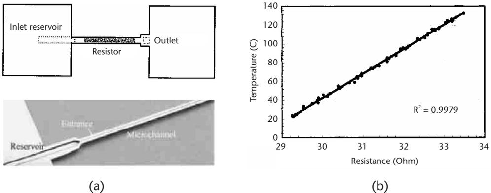
**Figure 10.5** (a) Microfabricated beam suspended silicon microchannels are used to investigate two-phase flow boiling behavior under constant heat-flux boundary conditions. Resistance temperature detectors (RTDs) and heaters were incorporated in the back side of the silicon beam by ion implantation, allowing for distributed temperature measurements and heating. (b) An RTD calibration curve shows the linear dependence between resistance and temperature [10].
