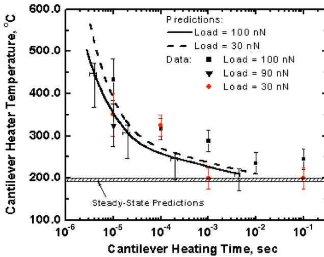
**Fig. 4 Prediction of the threshold conditions of time, temperature, and tip loading force required to produce a data bit for a 20 nm tip radius of curvature. The predictions compare well with data. The gray area shows predictions for near-equilibrium conditions.**
