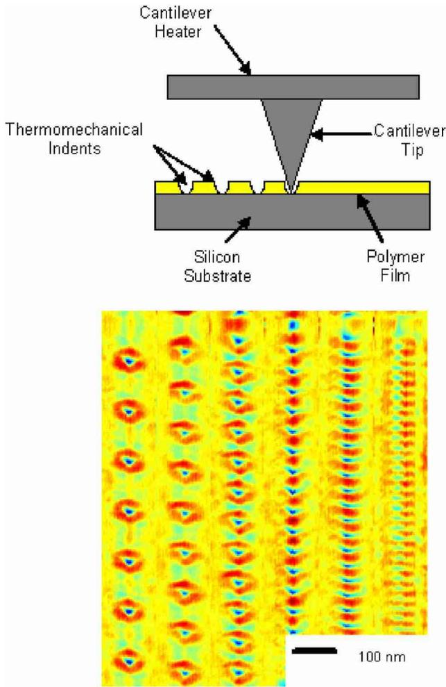
Fig. 1 Schematic of the bit-writing process and thermomechanically written indentations in polymer
