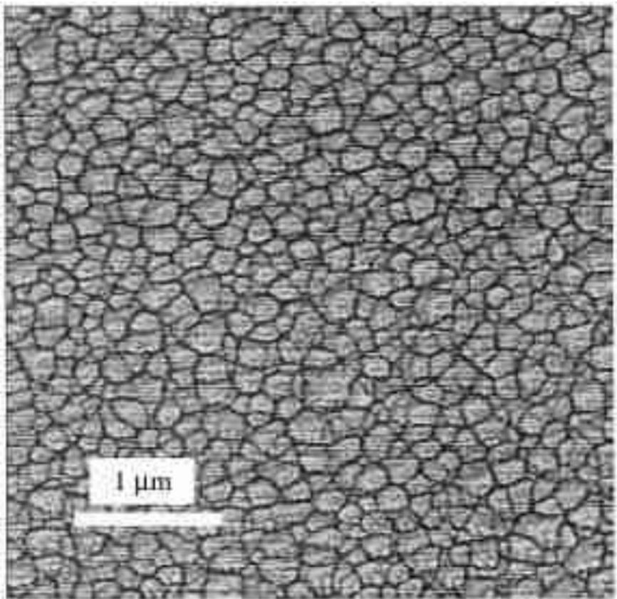
**Fig. 1.** Plan-view AFM image of polysilicon sample A showing the grains. The average grain size extracted using this image is 210 nm.
