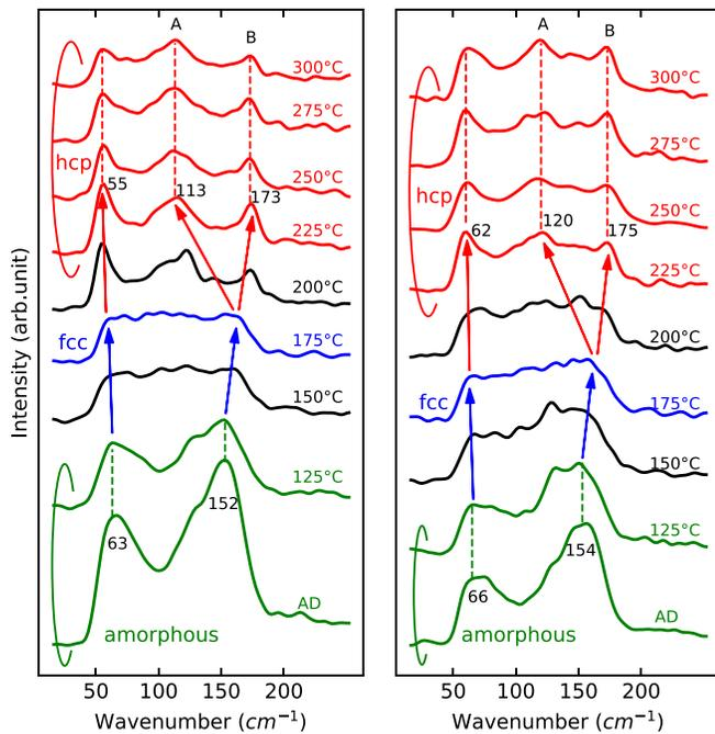
FIG. 3. Temperature dependence of Raman spectra of GST (left) and GST-Ni (right) from the as-deposited amorphous state to the hcp crystalline state after annealing at 300 °C. The vertical green and red dashed lines indicate the peak position in amorphous and hcp crystalline states, respectively. The solid arrows denote for peak shifting during phase transition. The black curves represent mixed transition states. All curves have been offset for clarity.
