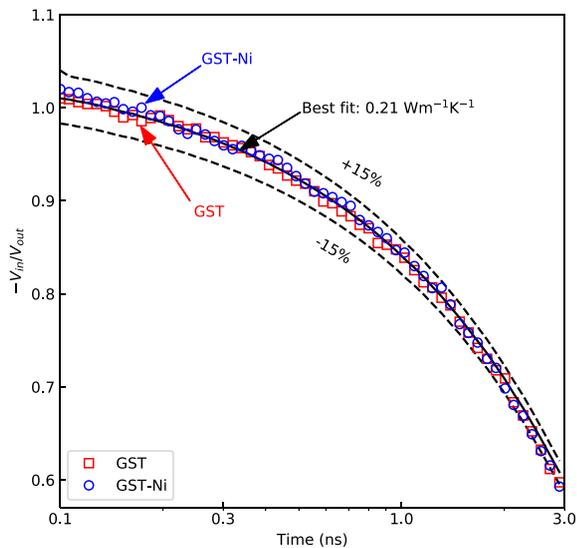
FIG. 4. Representative TDTR data for GST (red squares) and GST-Ni (blue circles) films. The black solid line denotes the best fit thermal conductivity of  $0.21 \text{ W m}^{-1} \text{ K}^{-1}$ . Black dashed lines correspond to  $\pm 15\%$  error bounds.
