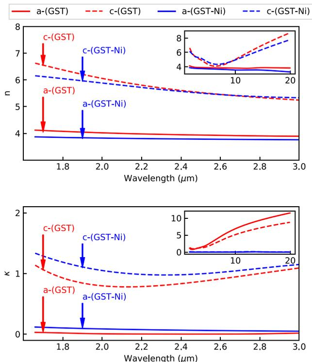
FIG. 5. Measured refractive index (top) and extinction coefficient (bottom) of GST and GST-Ni films in amorphous and crystalline states. The insets show  $n$  and  $\kappa$  in the spectrum up to  $20 \mu\text{m}$ .
