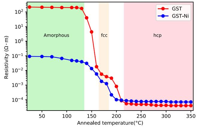
FIG. 1. Relationship between the resistivity and the annealing temperature of the as-deposited pure GST and GST-Ni (2%) films.
