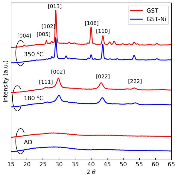
FIG. 2. XRD spectra of GST and GST-Ni samples for the as-deposited state (bottom) and after annealing at 180 °C (middle) and 350 °C (top). The curves have been offset for clarity.
