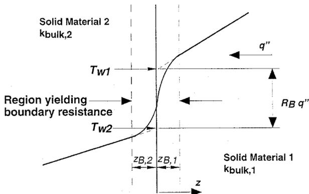
**Fig. 2** Schematic of the temperature distribution near solid-solid boundary. For acoustic-mismatch theories, the thicknesses  $z_B$  values are of the order of phonon mean free paths in the two materials. For incomplete contact theories, the  $z_B$  are comparable with the surface roughness. For the present study,  $z_B$  is governed by the thickness of highly disordered material.
