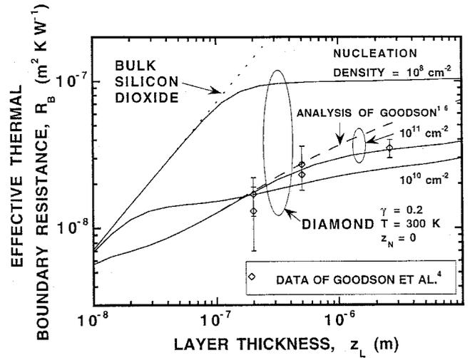
Fig. 5 Variation of the resistance normal to layers with nucleation density and film thickness.
