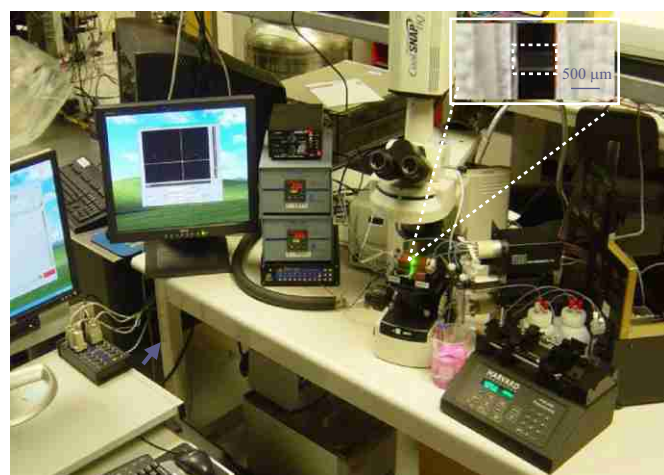
Fig. 4. A photograph of a TGF setup, showing an image of the microchannel in the inset (Ness, 2005).
