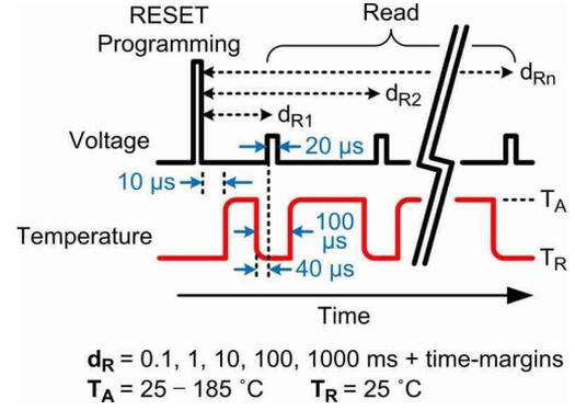
Fig. 4. Electrical pulse and temperature profile for  $R_{\text{RESET}}$  drift measurement. The measurement results are shown in Fig. 5. The cells are programmed and read at room temperature (25 °C). The cell resistances are read by small read voltage pulses at multiple delay times for reading, i.e.,  $d_R$ . The cells are annealed at various annealing temperature  $T_A$  between 25 °C and 185 °C by the Pt heater.
