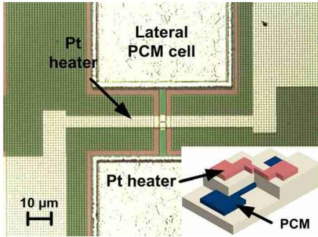
Fig. 1. Microscope image of an MTS. Pt heater is integrated on top of the lateral PCM cell. (Three-dimensional figure inset) The Pt heater overlapped region over narrow phase-change-material programmed region.
