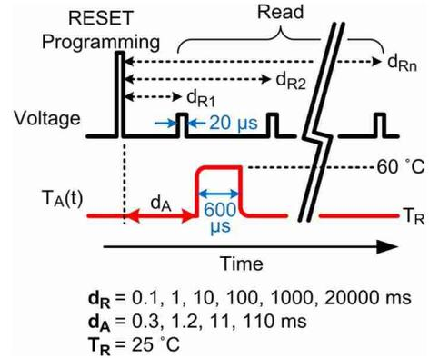
Fig. 7. Electrical pulse and temperature profile for  $R_{\text{RESET}}$  drift measurement. The measurement results are shown in Fig. 8. The cells are programmed and read at room temperature (25 °C).  $d_A$  and  $d_R$  are delay time for annealing and reading, respectively. The heat pulse is 600-μs long and 60 °C high.
