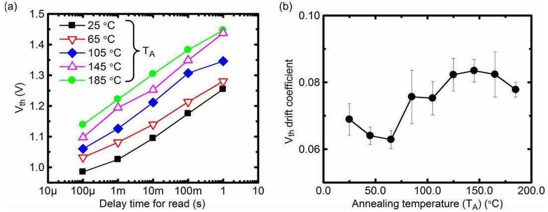
Fig. 10. (a)  $V_{th}(t)$  for various annealing temperatures  $T_A$ . (b) The  $V_{th}$  drift coefficient as a function of  $T_A$  calculated from (a). It shows the tendency to increase as  $T_A$  increases and agrees with the temperature dependence of the  $R_{RESET}$  drift coefficient. The cells are programmed and read at room temperature (25 °C). The measurement pulse details are shown in Fig. 9.
