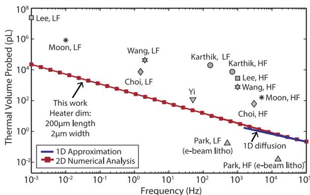
FIG. 2. Red line with squares: A 2D numerical analysis of the volume probed for the smallest heater ( $200\ \mu\text{m}$  length,  $2\ \mu\text{m}$  width) used in this work. Blue line: 1D diffusion approximation. Black points of various shapes: Comparison of the liquid volumes examined by previously published papers, calculated using the same method in this paper from their reported heater geometries and measurement frequency range from LF to HF.
