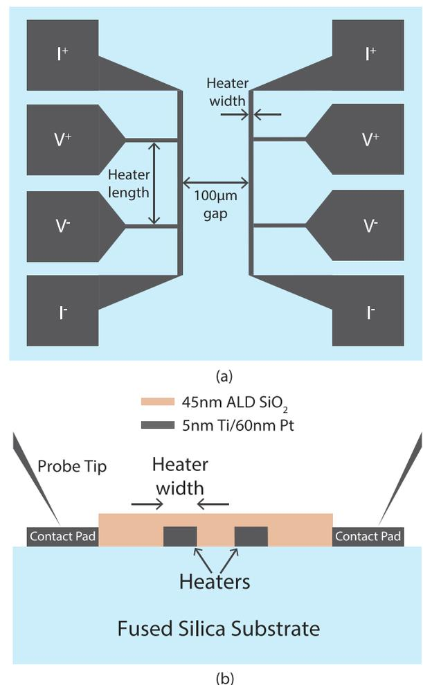
FIG. 1. (a) Top view of two isolated heater lines. (b) Cross-sectional view of device with 45 nm ALD  $\text{SiO}_2$  passivation layer etched away from metal contact pads to provide probe tip access.
