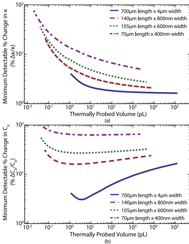
FIG. 7. Minimum detectable changes in  $\kappa$  (a) and  $C_p$  (b) vs. the thermally probed volume for the heater used in this work ( $700\ \mu\text{m}$  length by  $4\ \mu\text{m}$  width) and three smaller heater geometries of the same aspect ratio. Analysis uses a fused silica substrate and salt buffer fluid sample. Analysis is done using method explained in Eq. (8) using constant maximum current density to prevent electromigration effects.
