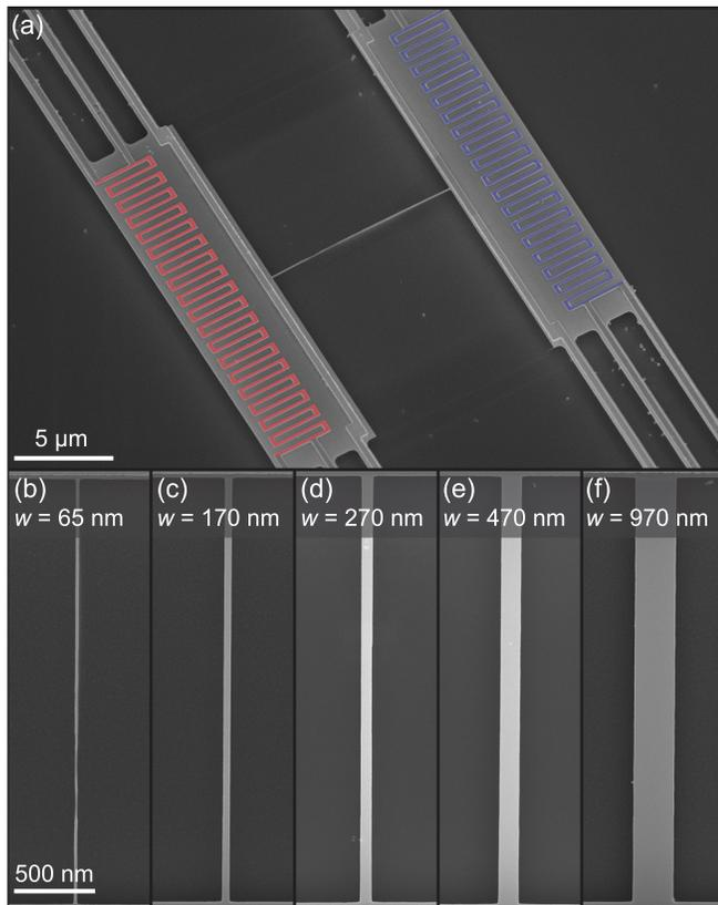
FIG. 1. (a) Overview of the “hot” and “cold” platforms for thermal characterization: false color on heater/thermometers. (b)–(f) Silicon nanobeams, with the width varied from  $\sim 65$  nm to  $\sim 970$  nm. The thickness is  $\sim 78$  nm for all samples.
