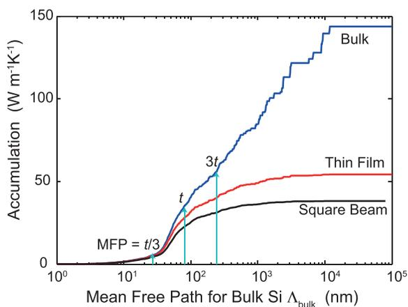
FIG. 3. Accumulation of thermal conductivity with a function of mean free paths for bulk silicon, a thin film with  $t$ , and a square beam with  $t = w$ , where  $t = 78$  nm. The accumulation function is calculated using Eqs. (3)–(5).
