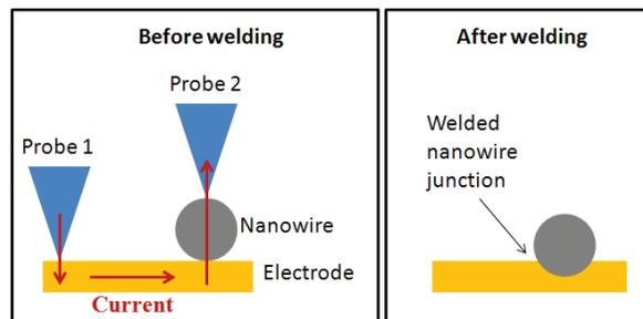
Figure 3. Schematic showing cross-section of nanowire welding process. One probe is placed on the metal electrode, and the other probe is placed on top of the nanowire. A voltage pulse is applied to the probes; the electrode melts locally at the electrode-nanowire junction. The local heating and the force of the probe on the nanowire reduce the contact resistance of the metal-nanowire junction.
