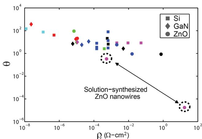
FIG. 5. The ratio of nanowire-internal to contact heat generation plotted as a function of reported contact resistivity for Si (■), GaN (◆), and ZnO (●) nanowire devices from various studies (Si,<sup>31,38–42</sup> GaN,<sup>33,43–46</sup> ZnO<sup>2,47–49</sup>). Nanowire material type is designated by marker type. Data from each source are differentiated by color as indicated in the references. Data from this work are circled.
