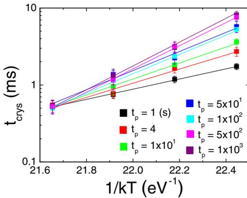
**Fig. 5.** (Color online) Crystallization time as a function of temperature ( $T$ ). The slope of the  $t_{crys}$  versus  $1/kT$  plot, which represents the activation energy, gets larger when we have a longer time interval  $t_p$ . The depicted lines are fits that show typical Arrhenius behavior, and the crystallization time was measured 5 times for each temperature to give statistical distribution.
