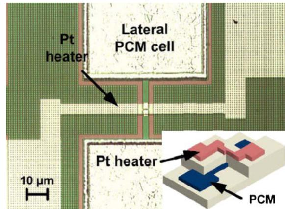
Fig. 1. (Color online) The top view microscope image of the lateral PCM cell bridged with the MTS platinum (Pt) heater. The inset shows the 3D bird's eye view. The  $\text{SiO}_x/\text{SiN}$  layer with thickness of about  $1 \mu\text{m}$  is used for passivation between the PCM cell and the Pt heater.
