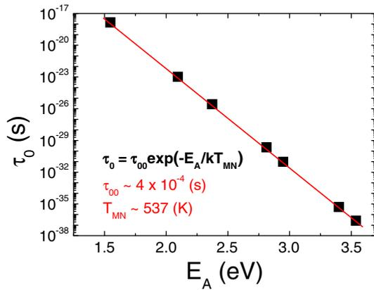
**Fig. 7.** (Color online) Meyer–Neldel plot of measured Arrhenius parameters of activation energy ( $E_A$ ) and pre-exponential factor ( $\tau_0$ ) and fit with extracted parameters of  $\tau_{00}$  and  $T_{MN}$ .  $\tau_{00}$  and  $T_{MN}$  are found to be  $4 \times 10^{-4}$  s and 537 K.
