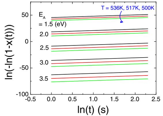
**Fig. 8.** (Color online) JMAK plot of  $\ln\{-\ln[1-x(t)]\}$  versus  $\ln t$  for different activation energy values of 1.5, 2.0, 2.5, 3.0, and 3.5 eV at  $T = 536$  (black), 517 (red), and 500 K (green).  $x(t)$  is the volume fraction of the crystallized material at time  $t$ .
