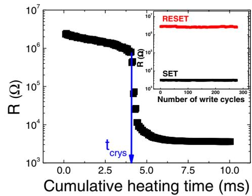
**Fig. 3.** (Color online) Crystallization due to thermal disturbances at  $T \sim 270 \text{ }^\circ\text{C}$ . Crystallization time ( $t_{\text{cryst}}$ ) is measured to be the cumulative heating time needed to form the first crystallization path within the amorphous region in the PCM cell. The inset shows the endurance characteristics with a high RESET/SET resistance ratio of  $\sim 1000$ .
