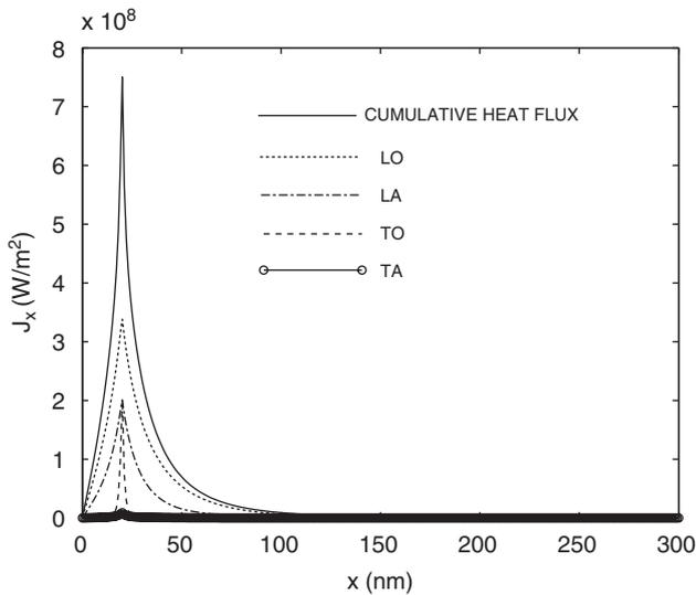
Fig. 9. A branch-wise break up of the far-from-equilibrium heat flux near a hotspot in a bulk device [19] shows the dominance of LO phonons.
