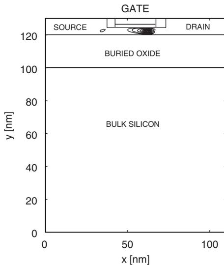
Fig. 1. The location of the heat source is shown in an ultra-thinbody SOI transistor operated at 1.2 V with a gate length of 18 nm [23]. The contours correspond to the spatial distribution of the heat generated inside the device and are equi-spaced at  $0.5 \text{ W/m}^3$  with a peak value of  $65 \text{ W/m}^3$  at the center.
