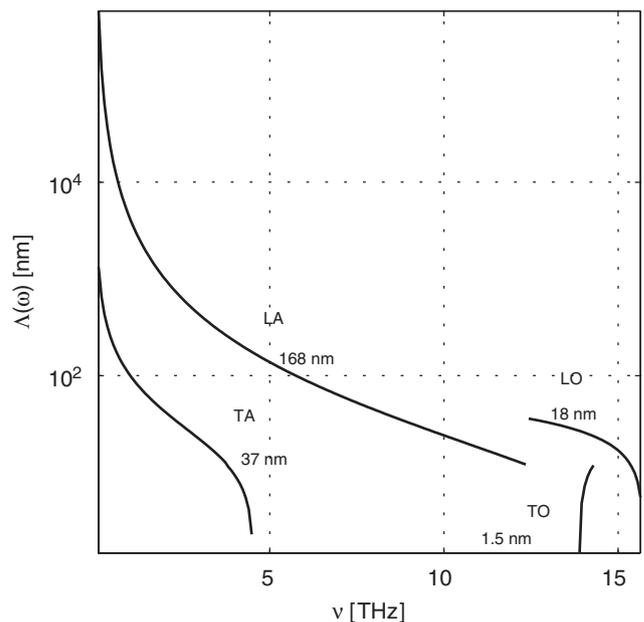
Fig. 11. The distribution of free paths in room temperature silicon as a function of phonon frequency and polarization is shown. The mean free path of phonons emitted by hot electrons in a device are also given for comparison. The use of a gray-body approximation for the heat source leads to large errors in predicting the magnitude of the hotspot effect.
