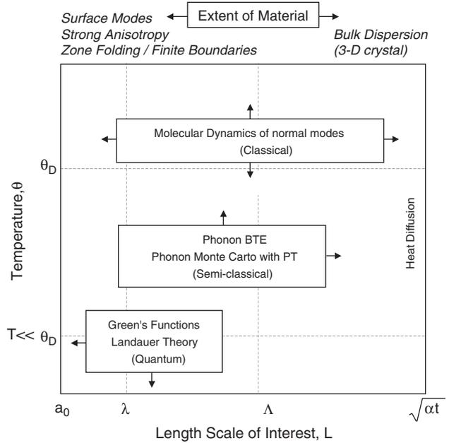
Fig. 3. Sub-continuum thermal modeling depends on the dimension of the system and the temperature. At dimensions comparable to the phonon wavelength and temperatures much smaller than the Debye temperature (bottom left), quantum mechanical nature is strongly manifest. At larger dimensions and room temperatures, a semi-classical approach is more pragmatic. PT in the figure stands for perturbation theory and  $a$  is the thermal diffusivity.
