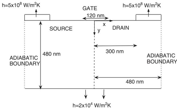
Fig. 6. The boundary conditions used in the device calculations are shown. The dashed line at the center is taken to be a line of symmetry. The hotspot is assumed to be semi-circular with a power density of  $5 \text{ W}/\mu\text{m}^3$ . Heat flows out through the bottom boundary with the heat transfer coefficient,  $h$ , as indicated. There is a second path for heat conduction, through the contacts shown at the top.
