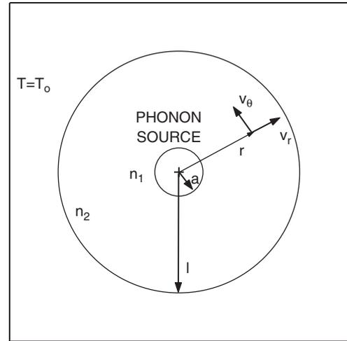
Fig. 7. The BTE is solved in a radial geometry with the source assumed to be confined within a radius equal to  $a$ . The solution is obtained in the two domains indexed as 1 and 2.
