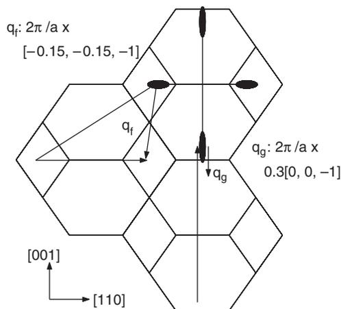
Fig. 4. The f- and g-processes are shown in a (110)-plane to identify the wave vectors of the involved phonons. The f-process phonon has the wave vector  $q_f$  and the g-process phonon has the wave vector  $q_g$  purely from geometry considerations.
