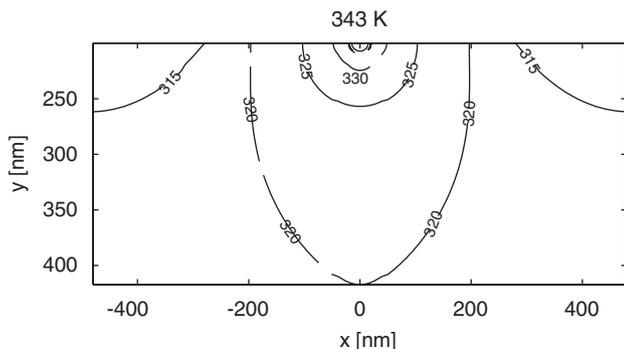
Fig. 10. The equivalent temperature field for phonon heat conduction from a device-like hotspot in bulk 90 nm geometry.
