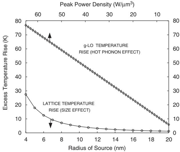
Fig. 12. The lower curve show the excess equivalent temperature rise in the lattice as a function of the heat source size. The source size is around 20 nm at the 90 nm node and is estimated to be around 4 nm for an 18 nm gate length device. The upper curve shows the excess equivalent temperature of the g-type longitudinal optical phonon as a function of the peak power density.
