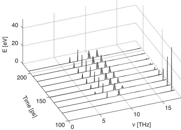
Fig. 5. Anharmonic phonon decay can be studied using atomistic simulations. The distribution of energy in the phonon spectrum is shown at various times during the decay of g-type longitudinal optical phonons at a hotspot with 50 eV energy.
