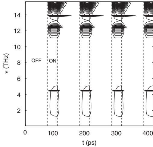
Fig. 14. Contours of the normalized phonon number density, spaced by 0.01, are shown as a function of frequency and time at  $x = 0$ . There is no phonon accumulation for a switching period of 100 ps with a duty cycle of 30%.
