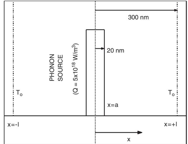
Fig. 13. A step-like phonon source symmetric about  $x = 0$  with a uniform power density of  $5 \times 10^{18} \text{ W}/\text{m}^3$  is considered as a sample calculation. The extent of the source,  $a$ , is taken to be 20 nm, consistent with device hotspots. A sink at 300 K is assumed to be at  $x = \pm l$  where  $l = 300$  nm.
