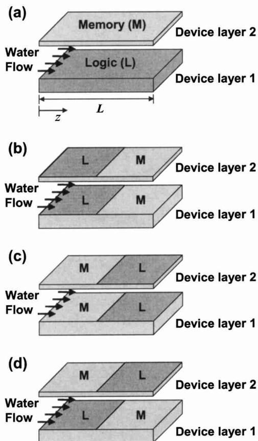
**Fig. 7 Two-layer 3D circuit layouts for evaluating the performance of microchannel cooling. The areas occupied by memory and logic are the same and the logic dissipates 90% of the total power consumption [53].**
