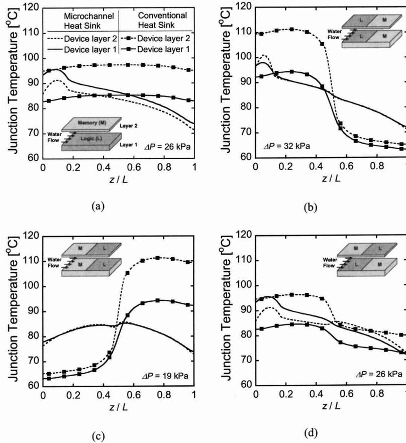
**Fig. 8 Comparison of junction temperatures in a two-layer stacked circuit for the cases of an integrated microchannel heat sink and a conventional heat sink. The total flow rate of the liquid water is 15 ml/min and the mass flux is  $1.36 \times 10^{-5}$  kg/s.**
