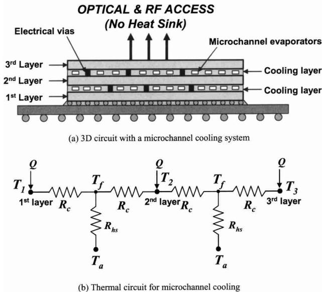
**Fig. 2 Conceptual schematic of a microchannel cooling network for a 3D circuit and the thermal circuit model. (a) 3D circuit with a microchannel cooling system. (b) Thermal circuit for microchannel cooling.**
