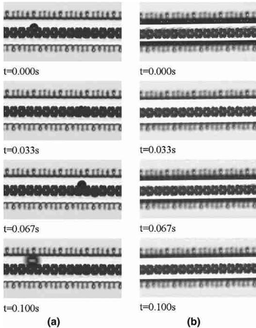
Fig. 8. Bubble nucleation and annular flow patterns in a 120  $\mu\text{m}$  wide, 52  $\mu\text{m}$  deep (72.5  $\mu\text{m}$  hydraulic diameter), enhanced-wall channel. (a) Bubble nucleation from cavities in the bottom of the channel. (b) Annular flow in the channel with varying liquid film thickness.
