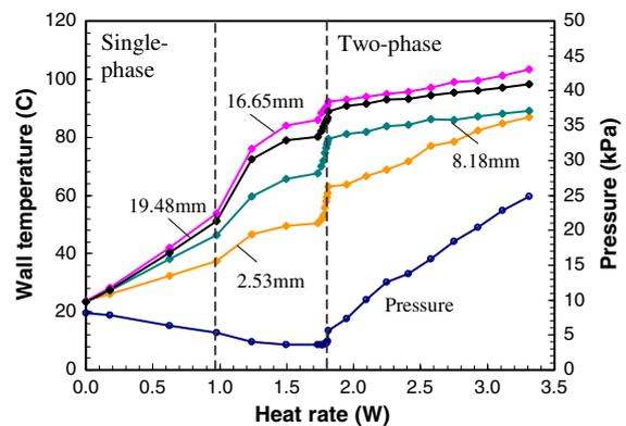
Fig. 4. Wall temperature change from four temperature sensors and global pressure drop as a function of input heat rate in a 100  $\mu\text{m}$  wide, 130  $\mu\text{m}$  deep (113  $\mu\text{m}$  hydraulic diameter) channel at 0.1 ml/min DI water flow rate. The numbers represent the distance between the sensor and the entrance of the microchannel.
