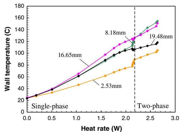
Fig. 9. Wall temperature change from four temperature sensors as a function of heat rate in a 50  $\mu\text{m}$  wide, 40  $\mu\text{m}$  deep (44  $\mu\text{m}$  hydraulic diameter) channel at 0.02 ml/min flow rate of 200 ppm TritonX-100 DI water solution. The numbers represent the distance between the sensor and the entrance of the microchannel.
