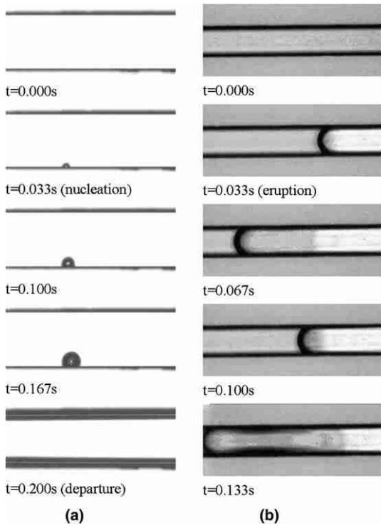
Fig. 3. Bubble nucleation mechanisms and two-phase flow regimes. (a) Bubble nucleation in a 250  $\mu\text{m}$  wide, 130  $\mu\text{m}$  deep (171  $\mu\text{m}$  hydraulic diameter) channel, with 0.5 ml/min DI water flow rate, 94–96  $^{\circ}\text{C}$  wall temperature; (b) Vapor eruption in a 50  $\mu\text{m}$  wide, 40  $\mu\text{m}$  deep (44  $\mu\text{m}$  hydraulic diameter) channel, with 0.02 ml/min DI water flow rate, 120  $^{\circ}\text{C}$  wall temperature.
