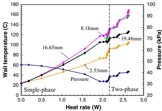
Fig. 5. Wall temperature change from four temperature sensors and global pressure drop as a function of input heat rate in a  $50\ \mu\text{m}$  wide,  $40\ \mu\text{m}$  deep ( $44\ \mu\text{m}$  hydraulic diameter) channel at  $0.02\ \text{ml/min}$  DI water flow rate. The numbers represent the distance between the sensor and the entrance of the microchannel. The short “plateaus” are artificial lines between input heat rate points, not measured temperature plateaus.
