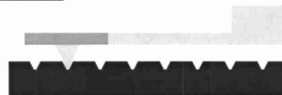
FIG. 1. Thermal reading of surface topography (see Ref. 3). The thermal resistance between the cantilever and the substrate varies as the cantilever tip follows the surface topography, producing a measurable change in the cantilever heating temperature.
