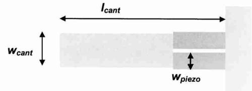
FIG. 2. Illustration of the thermal and piezoresistive cantilever geometry considered in this letter.
