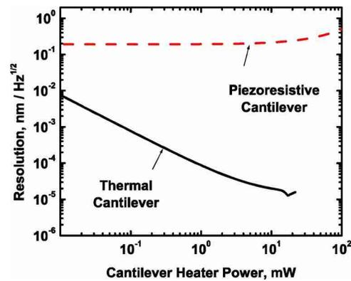
FIG. 4. Predicted minimum detectable feature size for the thermal cantilever and for the piezoresistive cantilever.
