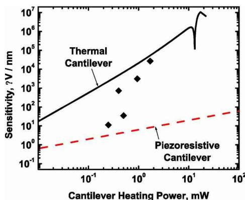
FIG. 3. Predicted voltage displacement sensitivity for the thermal cantilever and for the piezoresistive cantilever. Data are from previously published measurements of cantilevers close in design and operation to the model (Refs. 4 and 14).
