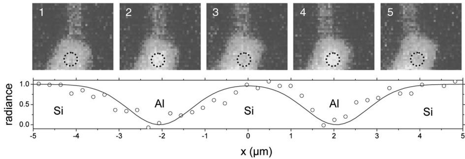
**Figure 2.** Sequence of radiance images of the microfabricated Si SIL as two  $1.0\text{-}\mu\text{m}$  Al lines separated by  $4.0\text{ }\mu\text{m}$  center-to-center are scanned beneath it. The two lines do not appear distinct in the CCD image but can be seen through the SIL in frames 2 and 4. The black dotted circle denotes the central region of the lens in each frame.
