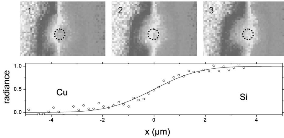
Figure 4. Sequence of radiance images of the microfabricated Si SIL as a Cu/Si edge is scanned beneath it.
