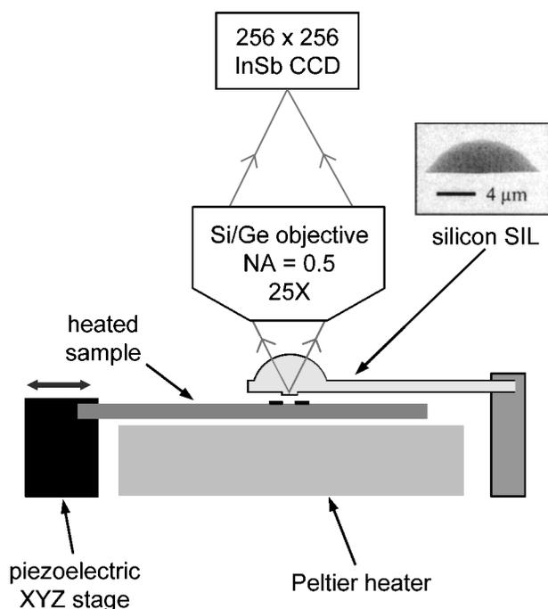
**Figure 1.** Experimental apparatus used for thermal imaging with the microfabricated Si SIL. A Peltier heater uniformly heats a sample held on a three-axis piezoelectric scanner. The SIL is fixed at the focus of the Si/Ge collection objective, and the sample is scanned below the SIL.
