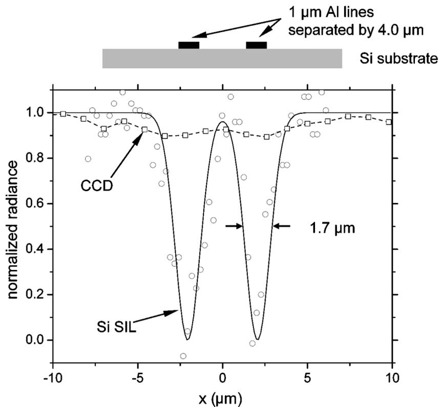
**Figure 3.** Line scans of two  $1.0\text{-}\mu\text{m}$  Al lines separated by  $4.0\text{ }\mu\text{m}$  center-to-center taken with the microfabricated Si SIL (circles) and with the InfraScope CCD (squares). The FWHM of a Gaussian profile fit to the data (solid line) is  $\lambda/2.9$  at  $\lambda = 5\text{ }\mu\text{m}$ .
