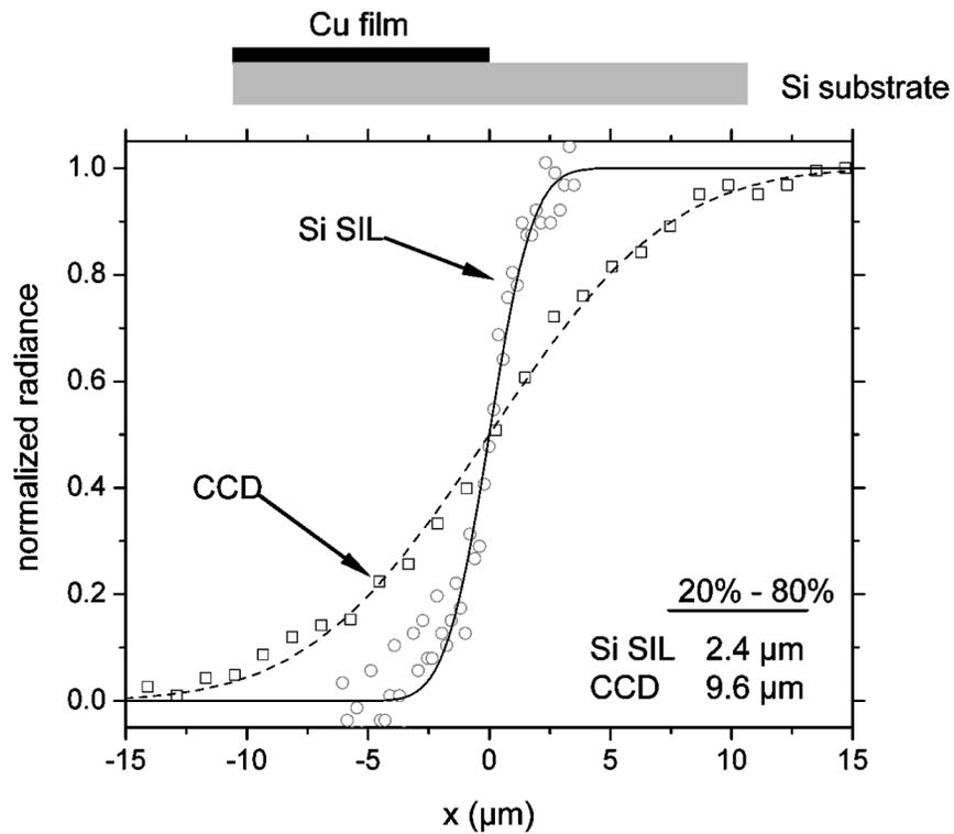
Figure 5. Edge scans of a Si/Cu edge taken with the microfabricated Si SIL and with the InfraScope CCD. The improvement in edge response is a factor of 4 over the CCD.
