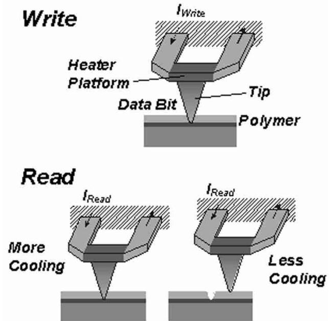
Fig. 1. Schematic of thermomechanical data writing and thermal data reading. The same cantilever can be used for both writing and reading. The heat transport mechanism for writing is distinctly different from that for reading, motivating concurrent optimization of the cantilever for both.
