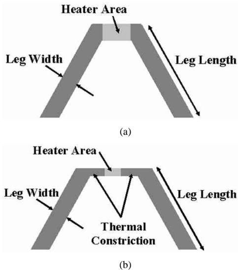
Fig. 6. Schematic of the basic cantilever "footprint." Cantilever Type A and Type B have the footprint of (a), and cantilever Type C has the footprint of (b). The thermal constrictions reduce the quantity of heat that flows along the legs of the cantilever, thus increasing writing speed and thermal reading sensitivity.
