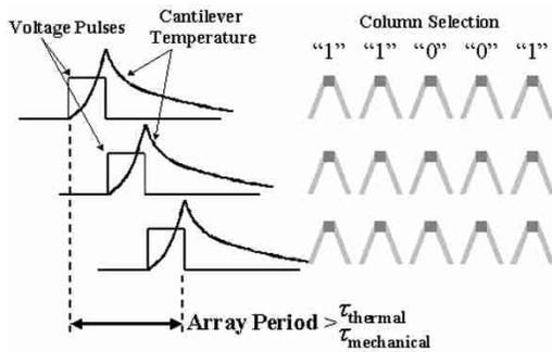
Fig. 10. The array operates with multiplexed row-by-row writing and reading [29]. Power is delivered for each row in a serial manner, and each cantilever will be selected for bit formation by connection of the electrical path along the column. A "1" refers to electrically switching the cantilever "on" for heating and bit formation; a "0" refers to keeping the cantilever switched "off" for no heating and no bit formation.
