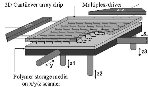
Fig. 3. The concept for a data storage device is to operate the cantilever array such that each of the cantilevers is in contact with a polymer data substrate. By scanning the cantilever array relative to the substrate and electrically selecting individual cantilevers from the array, high data rates and data capacity is possible.
