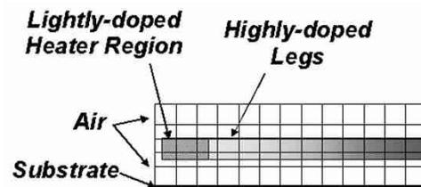
Fig. 5. The finite-difference simulation regime contains temperature nodes in and around the cantilever. The substrate can be added to the simulation as a boundary condition in order to predict cantilever operation during thermal data reading.
