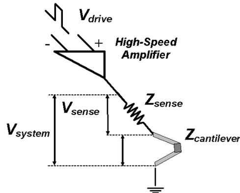
Fig. 4. High-speed electronics electrically drive and monitor the electrical response of the cantilever. The sense resistor is not needed in data writing, as data writing is accomplished in open-loop operation, but is required for thermal data reading.
