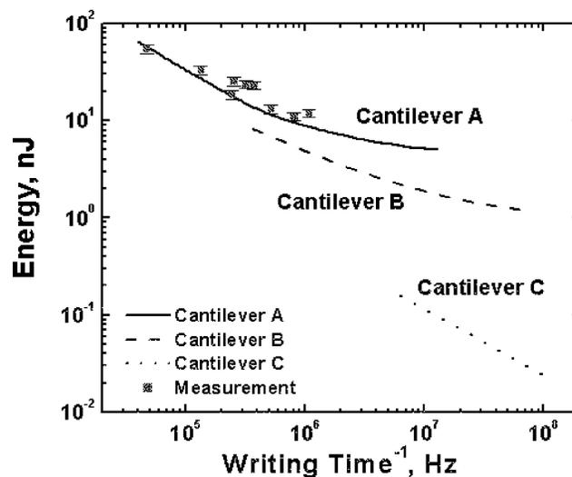
Fig. 8. Energy required to heat the cantilever to bit writing temperature as a function of the inverse of writing time. The inverse of writing time is close to the data writing rate. The electrical time constant of the measurement cantilever bond pad metal, limits measurement of Cantilever A.
