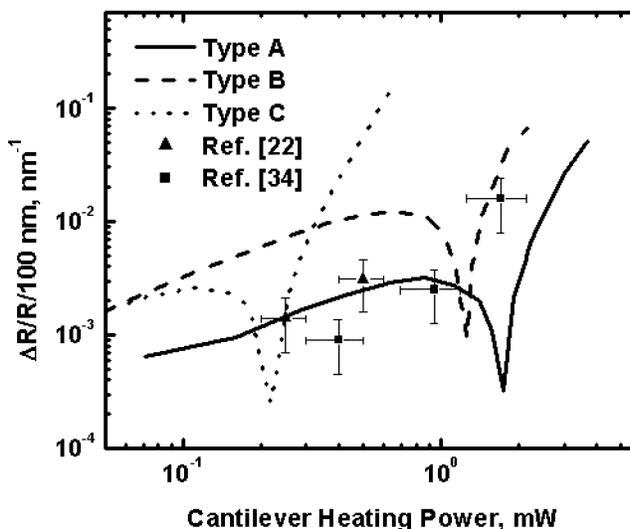
Fig. 9. Thermal data reading sensitivity as a function of cantilever heating power. The previously reported reading sensitivity was estimated in [21] and [29] for cantilevers with designs similar, but not identical to the Type A cantilever.
