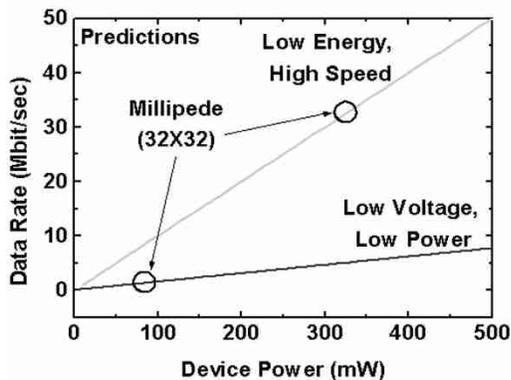
Fig. 11. Predictions for array operation of the Millipede Type A cantilever. The data rate can be varied by varying the cantilever driving voltage, which will correspond to a change in the power requirement. The circles represent operation of all 1024 cantilevers of the Millipede array shown in Fig. 2.
