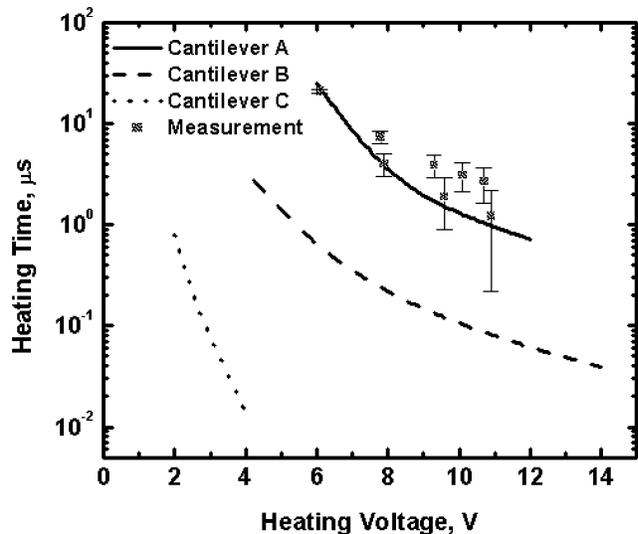
Fig. 7. Time required to reach the bit writing temperature as a function of voltage applied to the cantilever.
