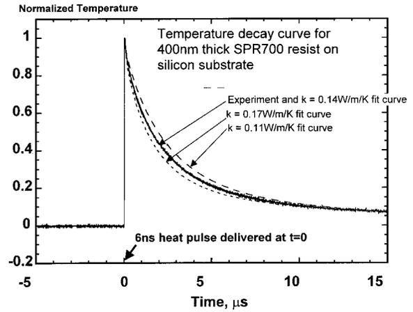
FIG. 3. Experimental temperature decay curve (from the experiments of unexposed SPR-700 resist) and corresponding curve fit of solution to heat conduction equation for the three different values of thermal conductivity  $k$ , clearly  $k=0.14$  W/m/K is the best fit of 400-nm-thick unexposed SPR-700 resist thin film on silicon substrate.
