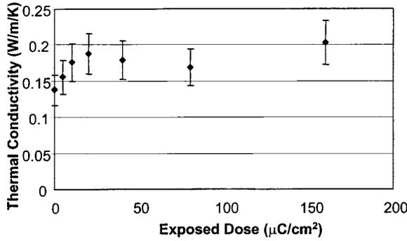
Fig. 4. Out-of-plane thermal conductivity of SPR resist following a variety of doses.
