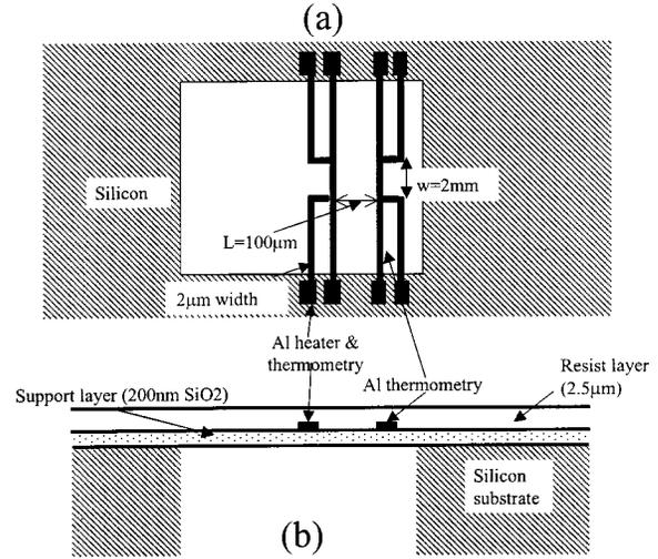
Fig. 5. (a) Top view and (b) cross section view of the structure for determining in-plane thermal conductivity.
