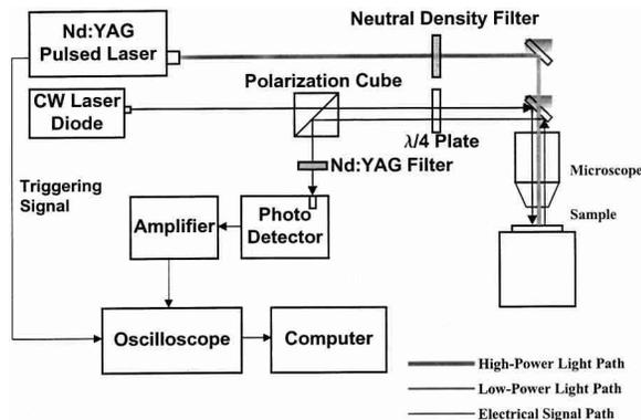
FIG. 2. Schematic of experiments for determining out-of-plane thermal conductivity.
