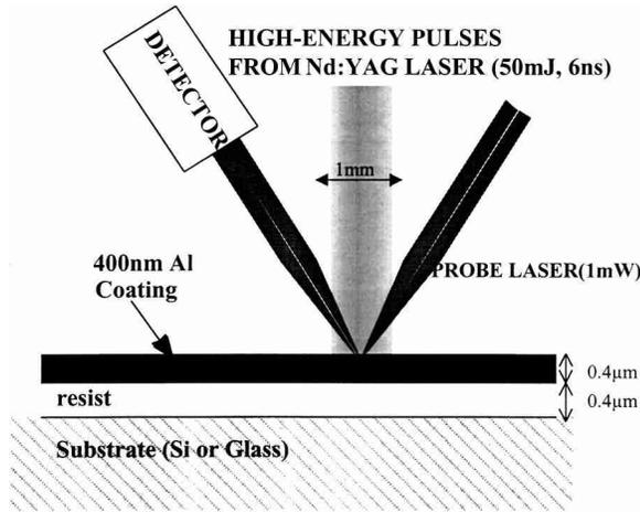
FIG. 1. Thermoreflectance method for determining the out-of-plane thermal conductivity of resist. Monitoring the reflectivity of the metal film allows us to follow the decay of surface temperature when we can determine the thermal conductivity of resist.
