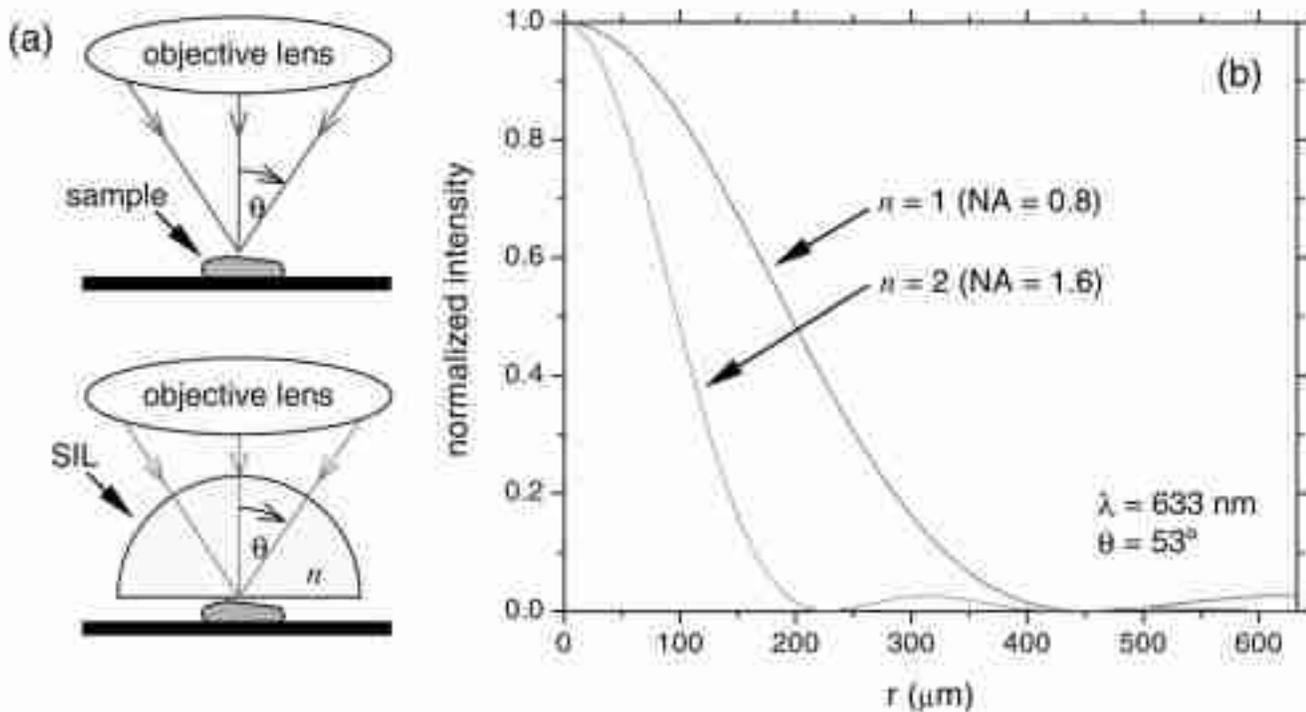
Fig. 1. Solid immersion microscopy. (a) Light is focused by an objective lens onto a sample in air with a maximum angle of incidence  $\theta$  and through a hemispherical SIL with index of refraction  $n$  and the same angle  $\theta$ . (b) The spot size in air with  $\lambda = 633$  nm illumination  $\theta = 53^\circ$  is decreased by a factor of 2 with a hemispherical solid immersion lens of  $n = 2$ .
