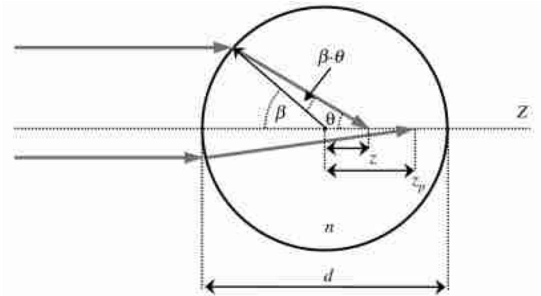
Fig. 8. Parallel rays incident on a spherical lens of diameter  $d$  and refractive index  $n$  showing spherical aberration. Rays are refracted at an angle  $\theta$  to the optical axis and focused to a point  $z$  from the geometrical center. Rays incident at a small angle  $\beta$  converge at the paraxial focus a distance  $z_p$  from the geometrical center.
