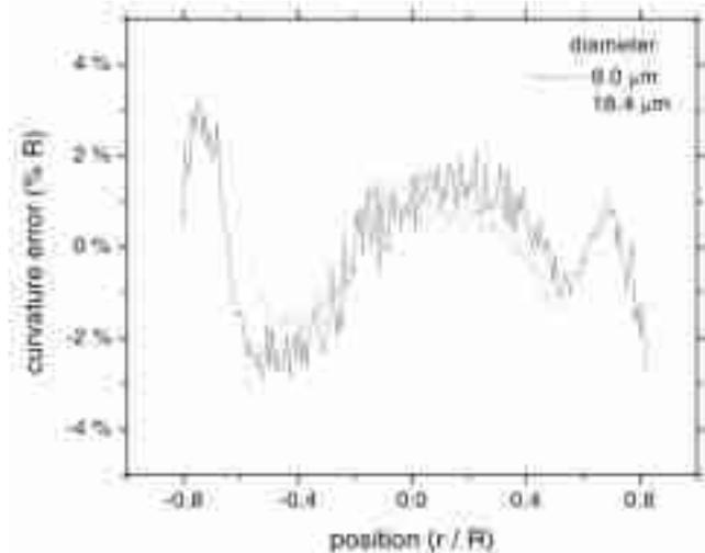
Fig. 7. Deviation in surface curvature of the SIL from spherical as a percentage of lens radius  $R$ . The surface topography of the lenses was obtained with an AFM.
