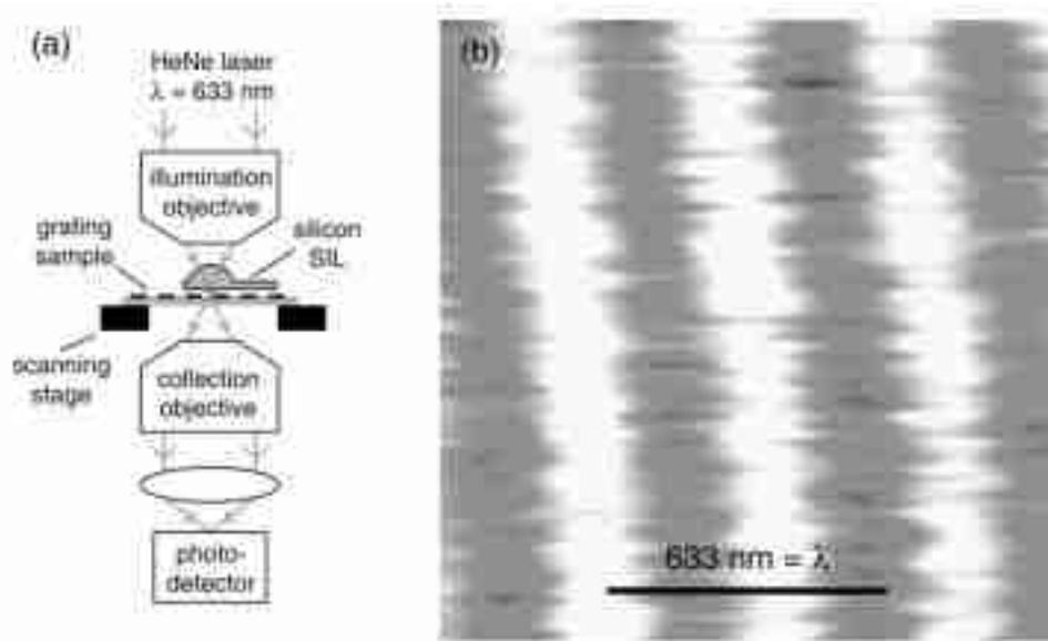
Fig. 10. Near-field imaging with the microfabricated Si solid immersion lens at a wavelength of  $\lambda = 633$  nm. (a) Experimental apparatus in which light from a HeNe laser is focused with a  $NA = 0.8$  illumination objective through the Si SIL onto the grating and imaged with a  $NA = 0.8$  collection objective and photodetector. (b) Two-dimensional image of a 200-nm linewidth grating taken in transmission with the scanned Si SIL showing resolution below the diffraction limit in air.
