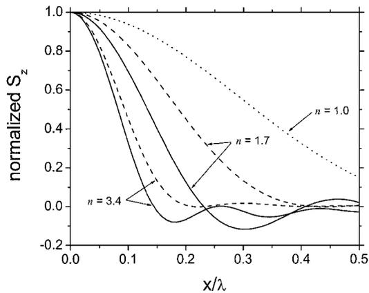
Fig. 4. Variation in spot size with index of refraction  $n = 3.4, 1.7$  in a Si microlens of diameter  $2\lambda$  for a NA of 0.8 at  $\phi = \pi/2$ . The solid curves show results from the converging wave model, and the dashed curves show the spots expected from vector diffraction theory.
