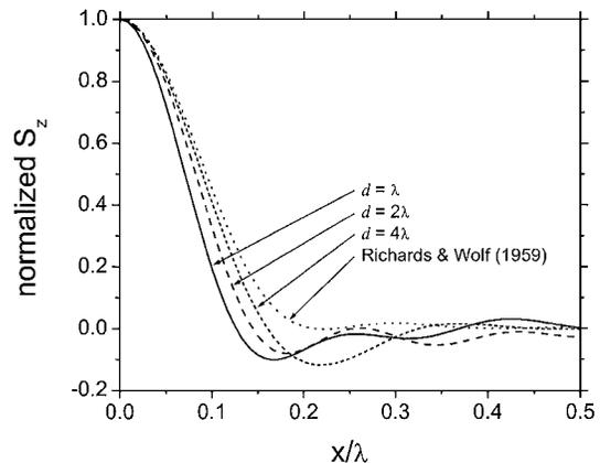
Fig. 2. Variation in spot size with Si microlens diameter for  $d = 4\lambda, 2\lambda, \lambda$  for a NA of 0.8 at  $\phi = \pi/2$ . The dotted curve shows the spot expected from vector diffraction theory.<sup>1</sup>
