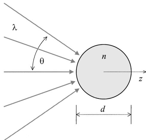
Fig. 1. Schematic of a spherical microlens of diameter  $d$  and index  $n$  illuminated by a converging wave of wavelength  $\lambda$  at a maximum angle  $\theta$ .
