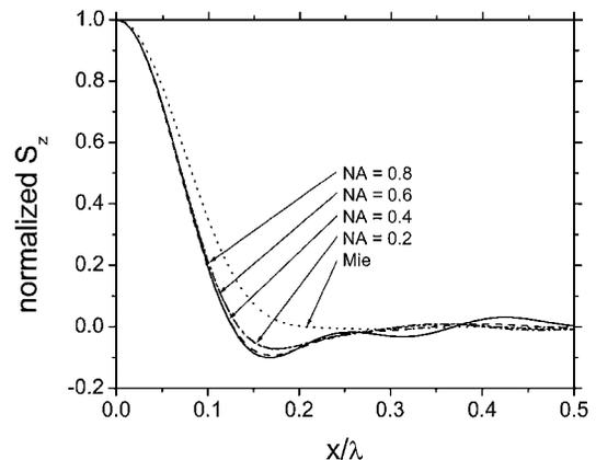
Fig. 3. Variation in spot size with illumination NA's of 0.8, 0.6, 0.4, and 0.2 in a Si microlens of diameter  $\lambda$  at  $\phi = \pi/2$ . The dotted curve shows the spot expected from Mie theory.
