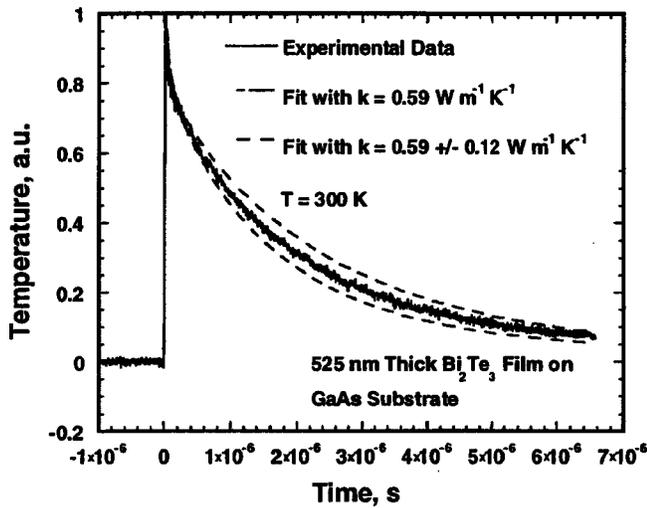
FIG. 3. The thermoreflectance signal and corresponding curvefit of the solution to the heat equation for the thermal conductivity measurement of Bi<sub>2</sub>Te<sub>3</sub> thin film of a thickness of 525 nm deposited on GaAs.
