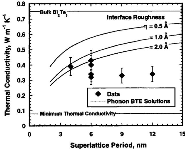
FIG. 4. Thermal conductivity of  $\text{Bi}_2\text{Te}_3/\text{Sb}_2\text{Te}_3$  superlattices of a function of period.
