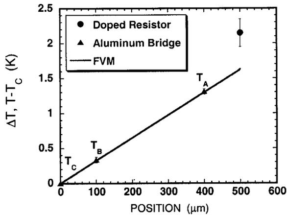
FIG. 2. Data and predictions for the temperature rise along the membrane. The temperature rises are referenced with respect to the temperature measured by the aluminum resistor *C*. Because of symmetry, the aluminum bridges provide three temperatures along what can be viewed as a single heat flow path for determining the membrane thermal conductivity.
