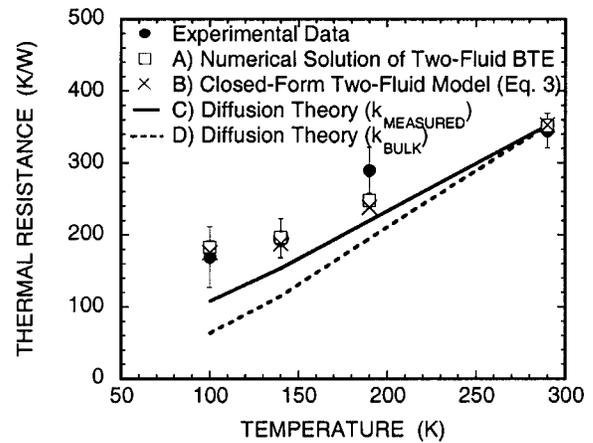
FIG. 3. Data and predictions for the membrane thermal resistance as a function of temperature. Prediction *A* is a numerical solution to the phonon Boltzmann transport equation with a simplified two-fluid model. *B* is a closed-form correction to diffusion theory based on the two-fluid phonon model. *C* and *D*, are based on diffusion theory, using the measured membrane thermal conductivity and the bulk thermal conductivity, respectively.
