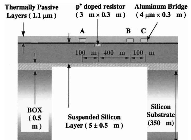
FIG. 1. Cross section of the experimental structure, which is micromachined from a SOI wafer. The doped resistor in the silicon membrane is used for heating and thermometry.
