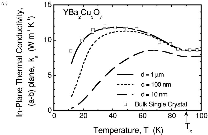
Figure 7 (Continued) Room-temperature thermal conductivities of single-crystal films and superlattices: (a) Predictions and data for conduction along SOI device layers (19). (b) Predictions of Chen (*heavy lines*) (33) for conduction normal to Si/Ge superlattices, compared with data of Lee et al (*filled circles*) (80). (c) Predictions of the in-plane thermal conductivity reduction due to electron and phonon scattering on interfaces in  $\text{YBa}_2\text{Cu}_3\text{O}_7$  films (38).
