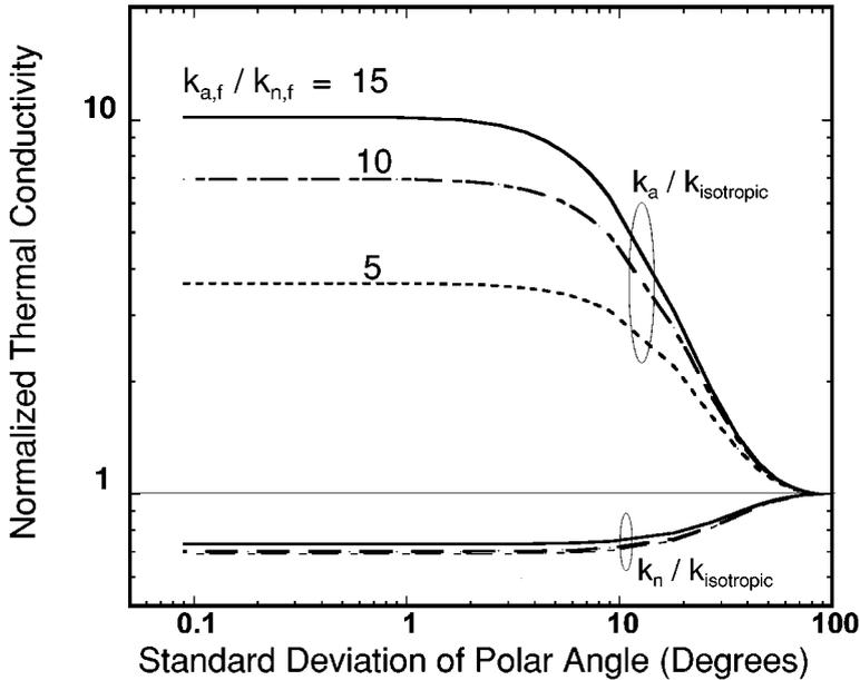
Figure 11 Predictions for the thermal conductivity anisotropy in fully amorphous polymer films (105).
