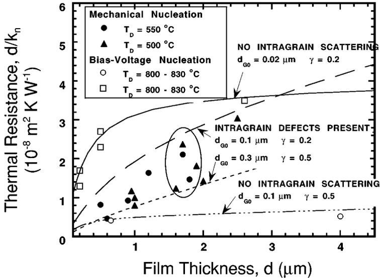
Figure 9 Dependence of the out-of-plane thermal resistance of polycrystalline CVD diamond films on the nucleation method and the film thickness (4). The grain size is assumed to vary linearly with the vertical coordinate,  $d_G = d_{G0} + \gamma z$ . The minimum grain size  $d_{G0}$  and spatial growth derivative  $\gamma$  are estimated from electron micrographs for the films. The predictions are based on the grain-boundary scattering strength model (64, 91).
