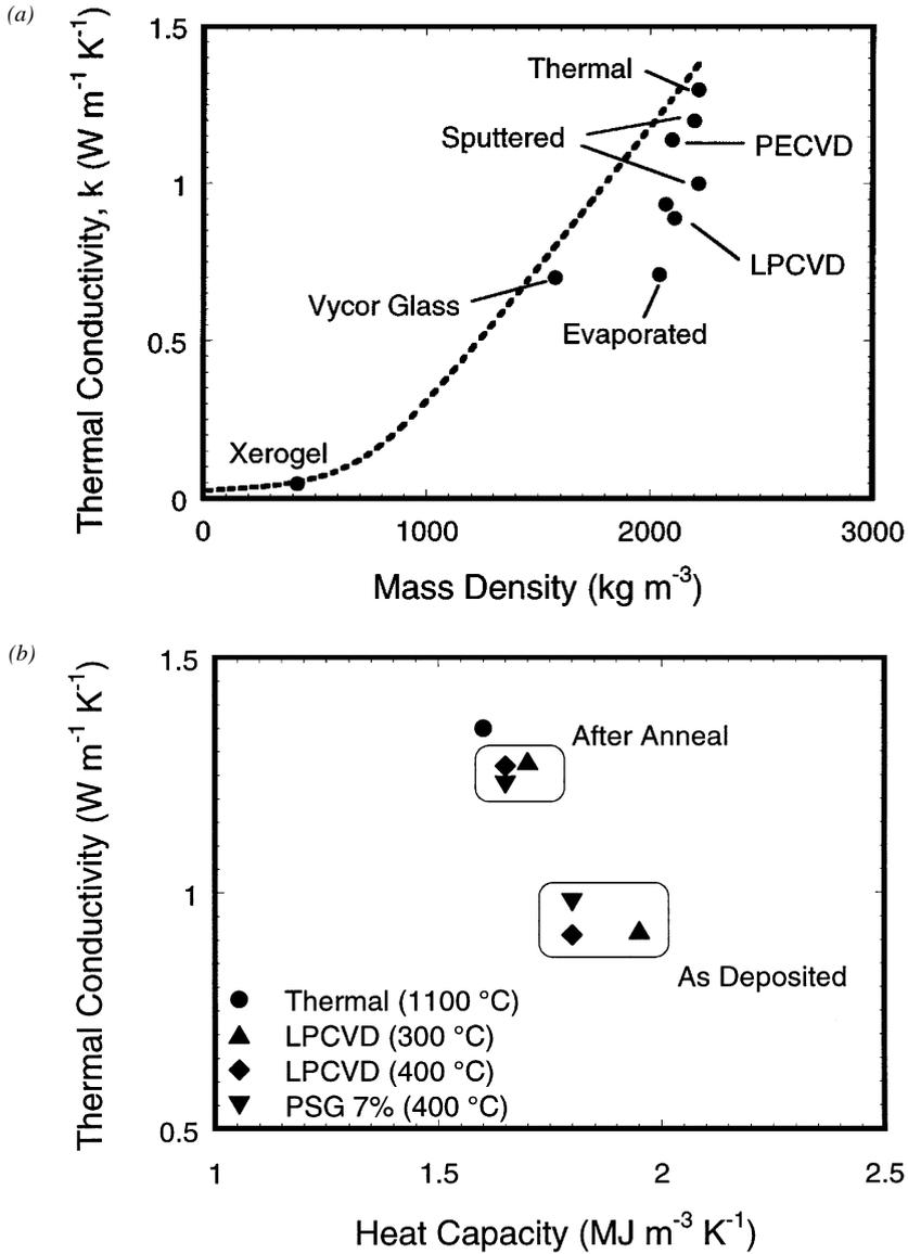
Figure 10 Process-dependent thermal properties of silicon dioxide films, which serve as representative fully amorphous films for the present review: (a) Density dependence of out-of-plane film thermal conductivity data (41, 97, 98) compared with predictions from the effective medium theory and data for porous silica glass (100) and a xerogel (101). (b) Variation of the volumetric heat capacity and the thermal conductivity with fabrication technique (26).
