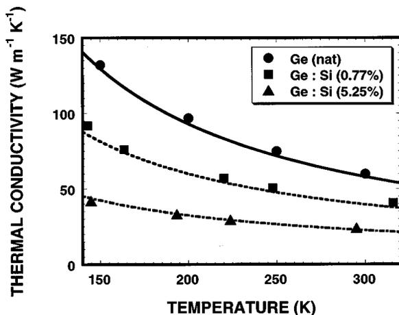
FIG. 3. Model predictions and previous data for the thermal conductivity of germanium crystals. The data for the isotopically enriched sample (Ref. 20), not shown here, are used to fix the model parameter  $B$ .
