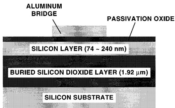
FIG. 1. Cross-sectional view of the thermal conductivity measurement structure employed in the present study.
