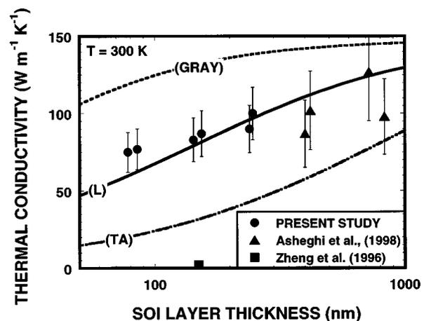
FIG. 2. Measured and predicted in-plane thermal conductivities of thin monocrystalline silicon layers at room temperature. The plot includes data from two previous studies (Ref. 6 and 10).
