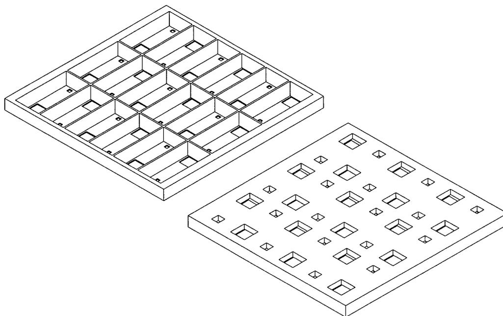
Fig. 2. Schematic of a micromachined silicon reaction vessel array for PCR. The top side (left) is sealed with 0.5-mm-thick Pyrex glass (not shown) through which TLC thermometry is performed. The working fluid is loaded through the square ports on the bottom side (right). The silicon component of the array (shown) has overall dimensions 11.0 mm  $\times$  11.2 mm  $\times$  0.7 mm.
