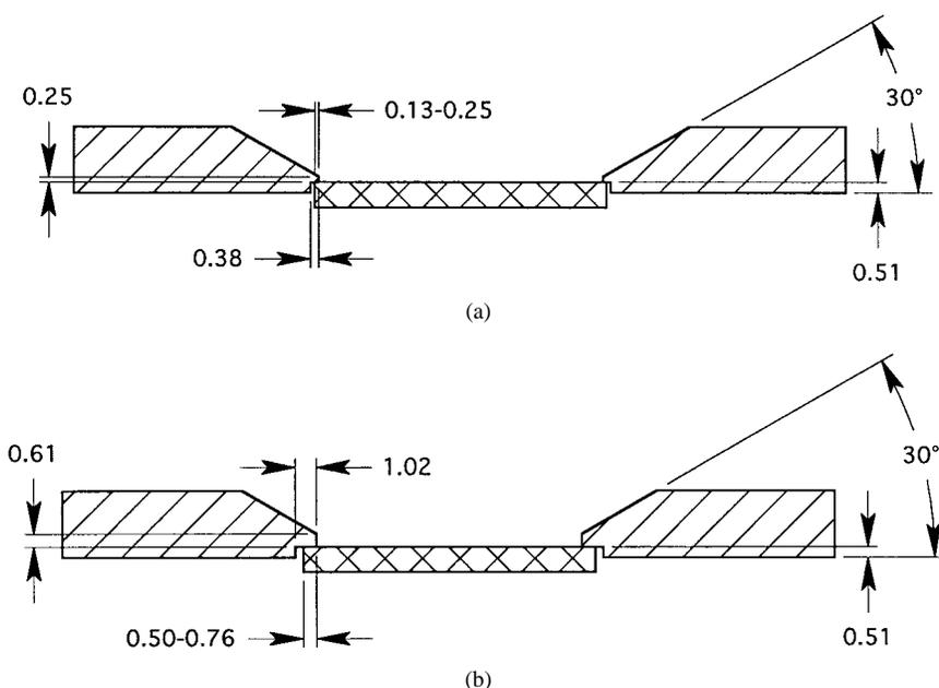
Fig. 5. (a) Section views of the small contact-area clamp and (b) large contact-area clamp. All dimensions are in millimeters. The increased contact surface of the large clamp and extra thickness near the contact surfaces allow larger heat flux to the clamp.
