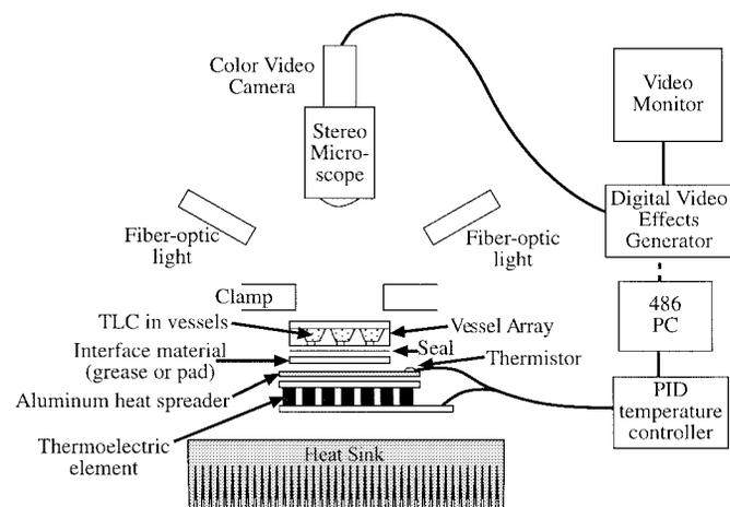
Fig. 4. Experimental apparatus for temperature mapping. The image of the TLC-filled vessels is passed to the digital effects generator, which adds an inset with time and temperature from the PC screen. The PID controller converts the thermistor resistance value to temperature.
