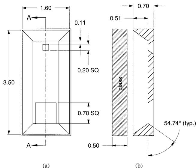
Fig. 3. Schematic of a single vessel showing the dimensions. (a) The top view shows the sizes of the loading and vent holes. The Pyrex glass plate shown in (b) is bonded to the silicon chip to seal the vessel on its top side. All dimensions are in millimeters.
