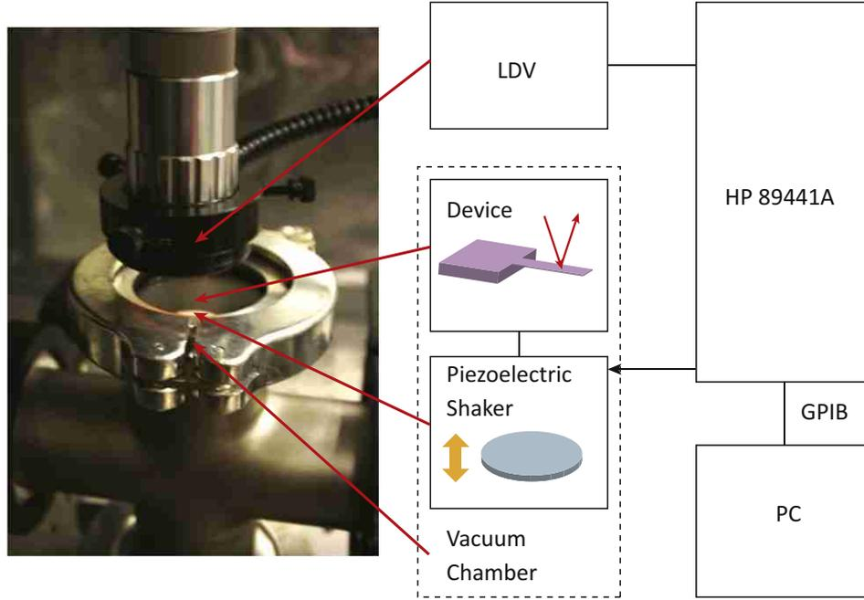
**Fig. 5 – Image and control diagram of the LDV system. A signal generator excites a piezoelectric disk around the cantilever’s fundamental resonant frequency. The resulting frequency spectrum from the LDV is recorded.**
