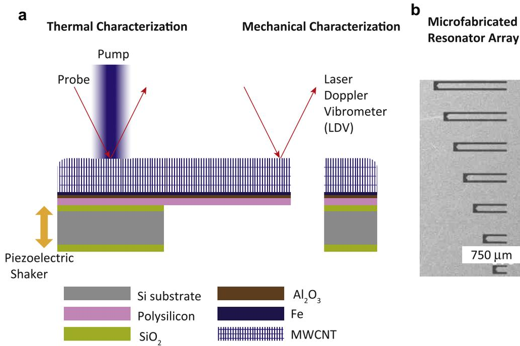
**Fig. 4 – (a) Schematic of the mechanical characterization structure. The structure allows simultaneous measurement of the thermal and mechanical properties using optical techniques. (b) SEM image of resonator arrays after the fabrication process, showing the variation in cantilever length to obtain various resonant frequencies.**
