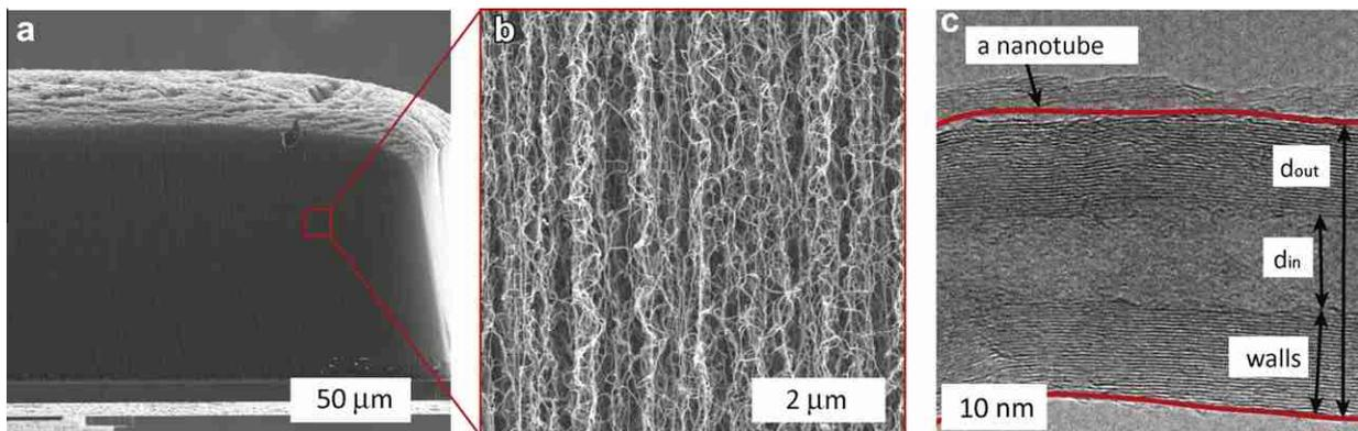
**Fig. 3 – (a) Scanning electron microscope (SEM) image of a 100  $\mu\text{m}$ -thick MWCNT film on a microresonator. (b) SEM image showing that the detailed morphology of a MWCNT film has a high degree of entanglement between the nanotubes. (c) Transmission electron microscope image of a single MWCNT taken from the film samples studied in this manuscript. The outer diameter of the nanotube is approximately 30 nm, the inner diameter is approximately 10 nm, and there are 25–30 walls.**
