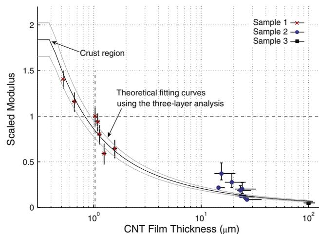
Fig. 9 – Theoretical fitting curves plotted against the scaled modulus to illustrate the thickness dependence of the elastic modulus of MWCNT films. The modulus is scaled here to reduce the effects of film density. The theoretical curves are calculated using the three-layer analysis over increasing middle layer thickness. The effective modulus significantly decreases with MWCNT film thickness as the relative impact of the high-modulus crust layer diminishes.
