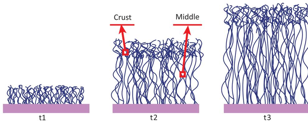
Fig. 8 – Schematics of the thickness-dependent structure of MWCNT films, with growth time increasing from  $t_1$  to  $t_3$ . The structure at  $t_1$  represents the formation of the crust layer with 400 nm. As the growth progresses ( $t_2$ ), a more aligned middle section is formed below the crust, which continues to grow from the base ( $t_3$ ).
