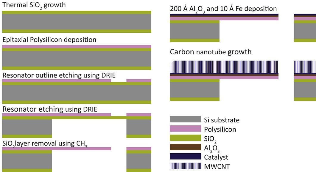
**Fig. 2 – Microresonator fabrication process and MWCNT film growth. Using this process, we can vary the SiO<sub>2</sub> and polysilicon thicknesses. The SiO<sub>2</sub> growth step can be substituted with commercial silicon on insulator substrates in the future. After the process, a completed wafer contains more than 3000 cantilevers.**
