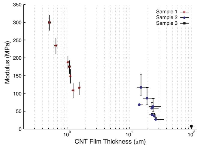
**Fig. 6 – Effective modulus of MWCNT films from three separate growths: samples 1 and 2 include films of thickness 0.5–1.6  $\mu\text{m}$  and 15–27  $\mu\text{m}$ , respectively. Sample 3, which contains one cantilever, has a thickness of 100  $\mu\text{m}$ . The film densities are 31–32  $\text{kg}/\text{m}^3$  (Sample 1), 55–56  $\text{kg}/\text{m}^3$  (Sample 2), and 29  $\text{kg}/\text{m}^3$  (Sample 3).**
