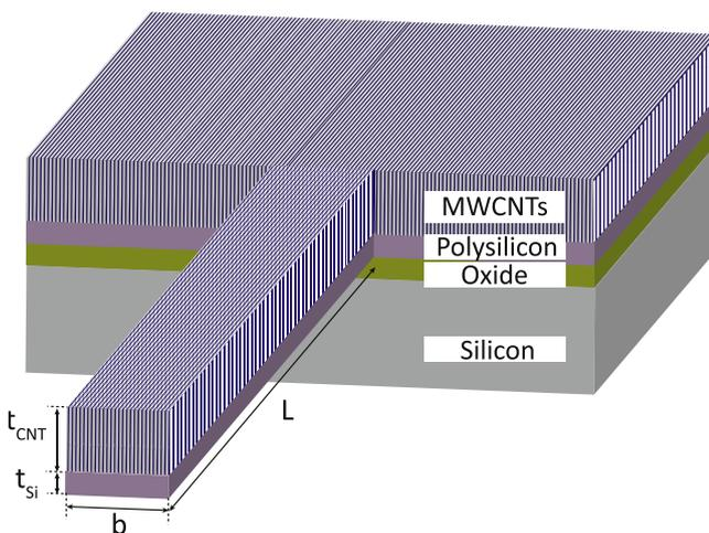
**Fig. 1** – Schematic of a polysilicon and MWCNT composite beam. Beam dimensions are varied to achieve a range of resonant frequencies. The film thicknesses of the MWCNT are varied to measure the thickness dependence.
