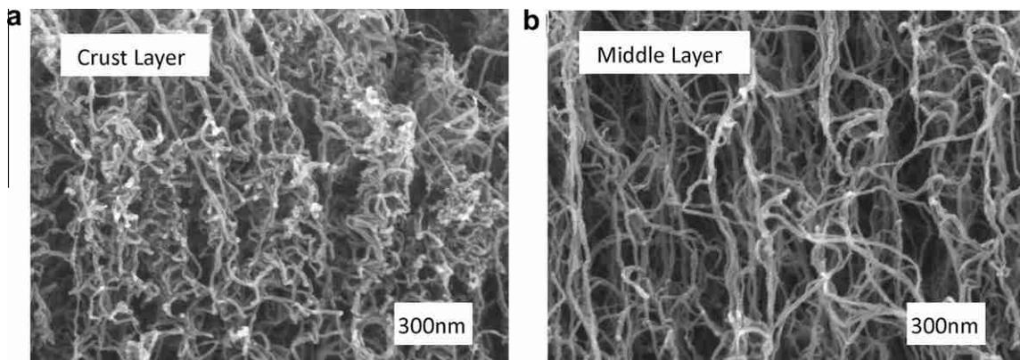
**Fig. 7 – SEM images of the crust and middle layer in a MWCNT film. (a) The crust layer exhibits more entanglement than the rest of the film. (b) The middle layer has straighter MWCNTs with lower density.**
