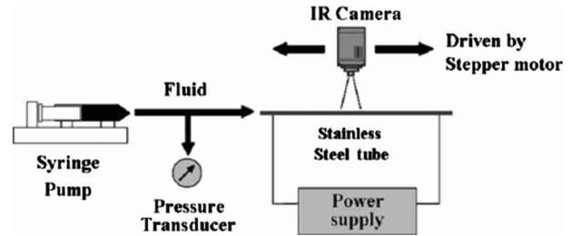
**Fig. 2 Experimental apparatus of convection and pressure drop measurement. infrared camera measures the outside wall temperature of stainless steel tube heated by power supply; pressure transducer measures the pressure drop in the microtube**
