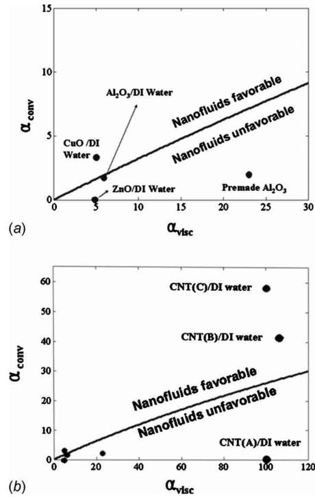
**Fig. 6 Effective viscosity and heat transfer augmentation data of seven different nanofluids: CNT(A)/DI water, CNT(B)/DI water, CNT(C)/DI water, CuO/DI water, Al<sub>2</sub>O<sub>3</sub>/DI water, ZnO/DI water, and premade Al<sub>2</sub>O<sub>3</sub>/DI water; all data are obtained from microtube experiment**
