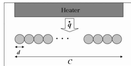
**Fig. 7 Multiple parallel channels with each diameter of  $d$ ; the total channel width is constant as  $C$**
