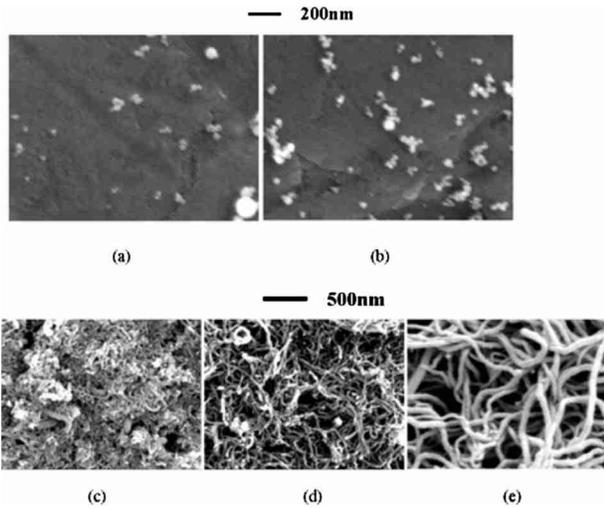
**Fig. 1 Scanning electron microscopy images of (a)  $\text{Al}_2\text{O}_3$  nanoparticles(40–50 nm), (b)  $\text{CuO}$  nanoparticles(13–37 nm), (c) multiwall CNT(A) (10–30 nm and 1–10  $\mu\text{m}$ ), (d) multiwall CNT(B) (10–30 nm and 0.5–50  $\mu\text{m}$ ), and (e) multiwall CNT(C) (40–60 nm and 5–15  $\mu\text{m}$ ) after evaporation of deionized water in nanofluids**
