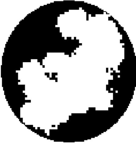
FIG. 5. Binary version of aggregate from SEM image. The particle volume fraction in the aggregate is estimated from this image to be 0.51.
