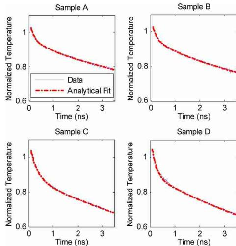
Fig. 2. Representative thermal traces and data fits at 30 °C for each of the four samples. Each thermal decay trace is the average of ten traces.
