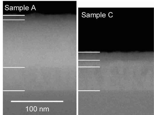
Fig. 1. Cross-sectional SEM images of two measured samples. From the top, the layers are TiN, fcc GST, TiN, and Si. Approximately 53-nm layers of Al were evaporated on these structures and measured using AFM after the SEMs were taken. The white lines are intended as a guide for distinguishing between layers.
