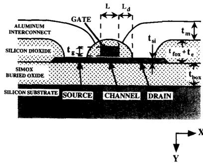
Fig. 2. Cross-sectional view of a completed SOI MOSFET. The device dimensions are given in Table I.
