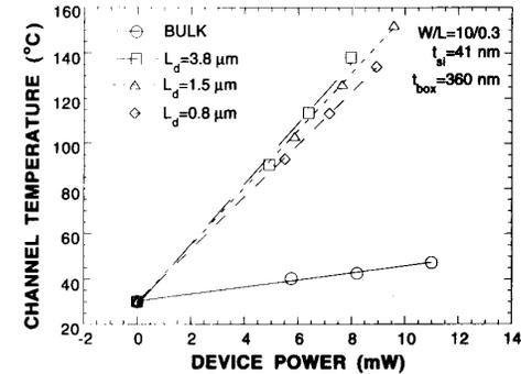
Fig. 7. Channel temperature versus power for several channel-metal contact separations.
