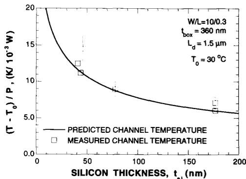
Fig. 9. Prediction of the channel-substrate thermal resistance as a function of source and drain thicknesses.
