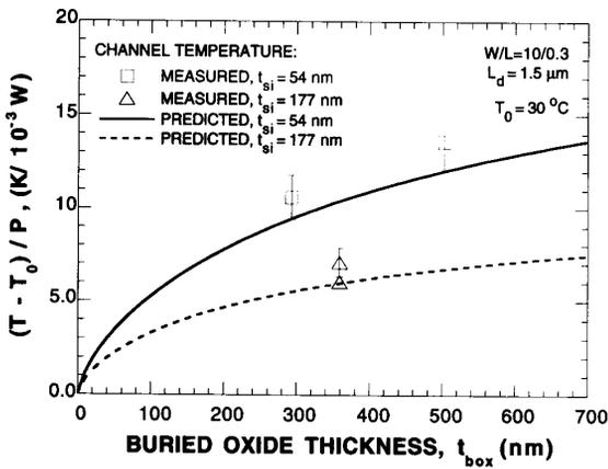
Fig. 11. Prediction of the channel-substrate thermal resistance as a function of buried oxide thickness.
