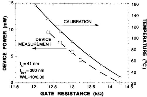
Fig. 4. Calibration and device measurement data for a typical SOI device.
