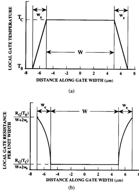
Fig. 3. (a) Assumed temperature profile along the gate electrode (in the Z direction) of an SOI MOSFET. (b) Corresponding gate electrode resistance per unit width (in the Z direction) of an SOI MOSFET.
