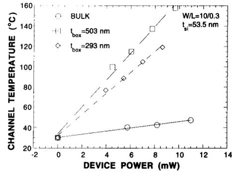
Fig. 6. Channel temperature versus power for several buried oxide thicknesses.
