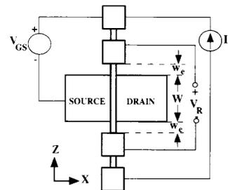
Fig. 1. Top-view of the experimental test structure for temperature measurement.  $W$  is the channel width and  $w_c$  is the region between the device edge and the gate contact pad.
