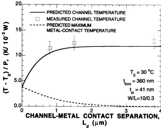
Fig. 10. Prediction of the channel-substrate thermal resistance as function of channel-metal contact separation.
