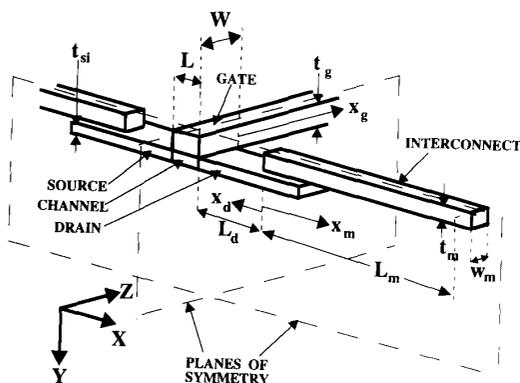
Fig. 8. Schematic of the fin geometry in the thermal model of an SOI MOSFET.
