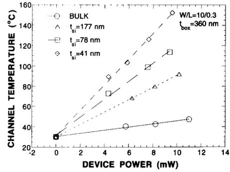
Fig. 5. Channel temperature versus power for SOI devices for several silicon thicknesses and a bulk device.
