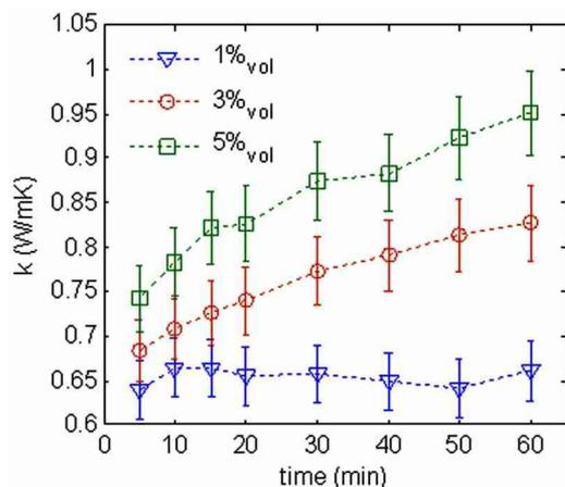
FIG. 3. (Color online) Time dependence of average thermal conductivity for varying concentration in nanofluid consisting alumina particles in water.
