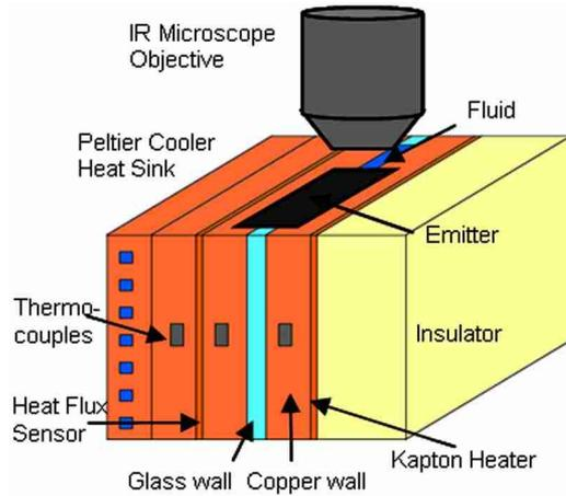
FIG. 1. (Color online) Schematic of IR microscope experimental setup with nanofluid held between copper plates. A heat flux is applied across the nanofluid with a thin Kapton heater, measured on the opposite side with a heat flux sensor, and dissipated into a Peltier cooler and heat sink. The temperature is monitored with thermocouples on the copper plates.
