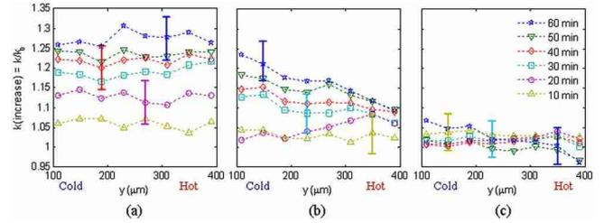
FIG. 2. (Color online) Time dependence of the full field thermal conductivity increase of a nanofluid consisting of alumina particles in water in a temperature gradient for volumetric concentrations of (a) 5%, (b) 3%, and (c) 1%. While the experimental uncertainty makes it impossible to extract conclusions for the case of 1% concentration, the trends observed for the other two concentrations are significant beyond the uncertainty.
