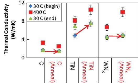
Fig. 1. Thermal conductivity of the single-layer electrode samples. The red arrows indicate the change of room temperature conductivity between the as-deposited and postannealed samples. Error bars are due to uncertainty in sample thickness.
