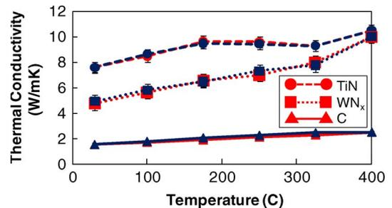
Fig. 2. Thermal conductivity of the postannealed single-layer samples. The (light) red points indicate the heating curve, and the (dark) blue points indicate the cooling curve. Hysteresis effects are not visible for these samples.
