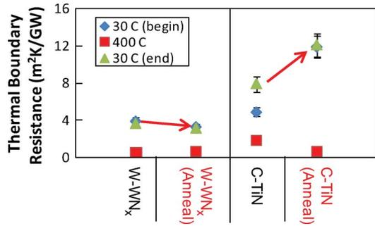
Fig. 3. TBR electrode multilayer samples. The red arrows indicate the change of room temperature TBR between the as-deposited and postannealed samples. Error bars are due to uncertainty in the thickness of the electrode films.
